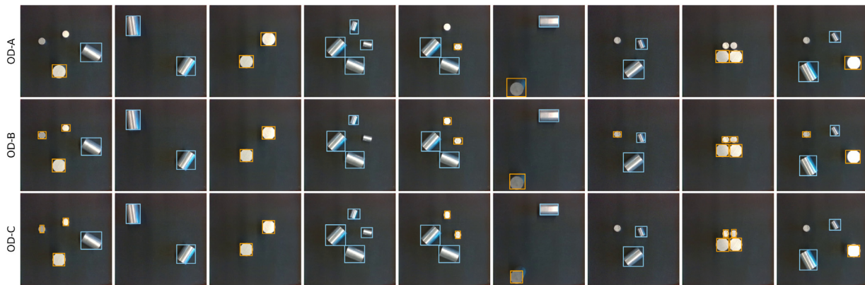
Fig. 10. Object detection results as bounding boxes for the cylinder in the lying pose (blue) and upright pose (orange). (For interpretation of the references to colour in this figure legend, the reader is referred to the web version of this article.)
