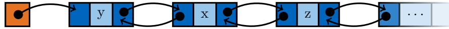
Figure 2.1: Example of an unordered list. Serving a request to item z requires linearly searching through the list starting from the beginning at y . Searching item z incurs cost 3 given by its list position.
