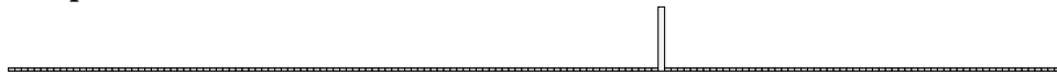
Figure 4.5: A surprisingly problematic input set \mathcal{J} for random-order arguments. A gigantic job carries almost all the processing volume; other jobs are negligible. All permutations of \mathcal{J} look basically the same. Such “simple” inputs need to be excluded before undertaking a random-order analysis.
