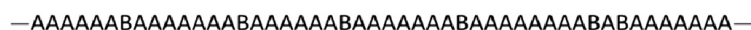
Fig. 2. Sequence of monomers A and B in a copolymer obtained when r_1 > 1 and r_2 < 1 .
