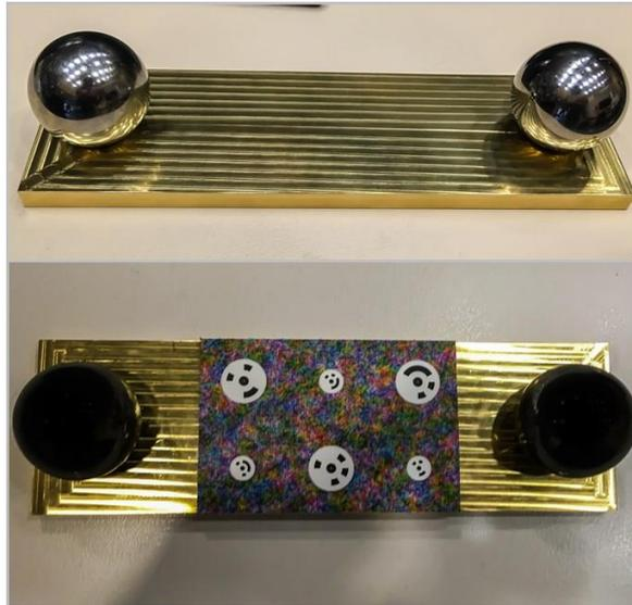
**Figure 14:** Sphere plate before and after its preparation
