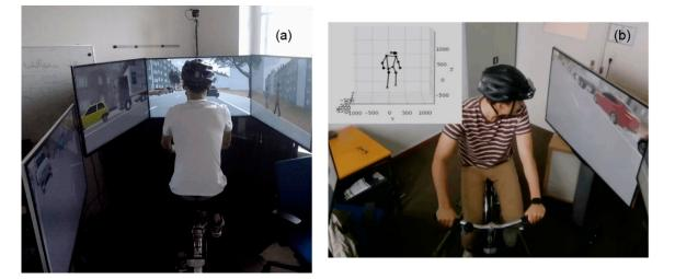
**Figure 3.** Setup of the currently used bicycle simulator with (**a**) depth camera of the type Intel<sup>®</sup> RealSense<sup>TM</sup> D435 and (**b**) detection of skeletal information and head-movement tracking.
