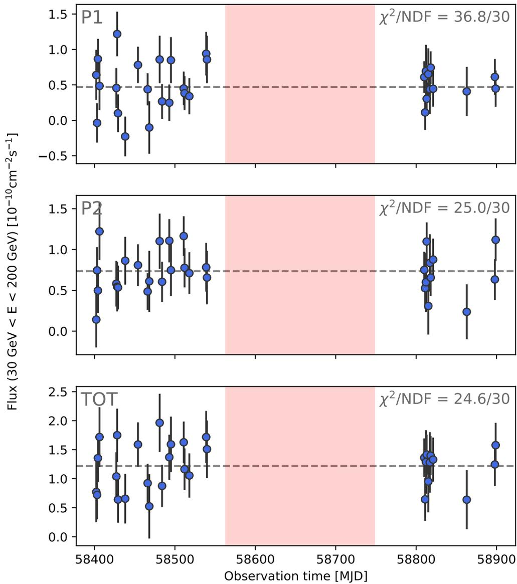
**Figure 5.10:** Nightly flux in the 30 GeV to 200 GeV energy range of the P1 (top panel) and P2 (middle panel) emission, as well as the total sum of the two (bottom panel), plotted against time in MJD. No significant deviation from a constant can be seen ( $\chi^2$  test) for any of the components. The red shaded area corresponds to the summer period during which the Crab pulsar is not observable from La Palma (from March to September).
