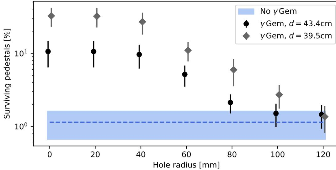
**Figure 4.12:** Surviving pedestals in a sample of Geminga data, as a function of the radius of the exclusion circle around the star Alhena and its distance  $d$  from the center of the camera. The blue band shows the same for a position not affected by Alhena. To recover the same performance, a 100 mm and 120 mm hole has to be cut, respectively.
