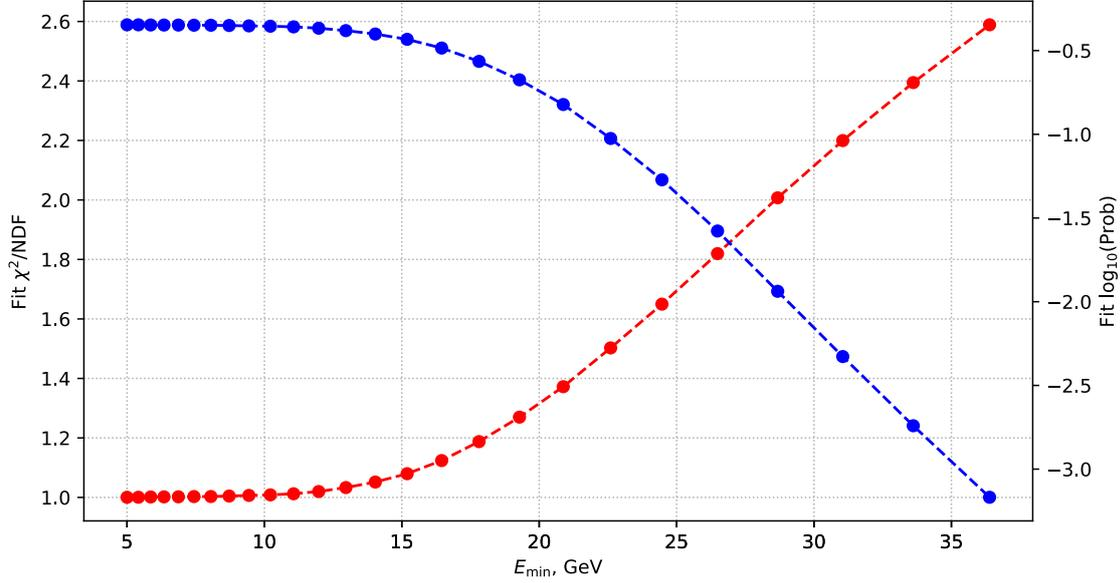
**Figure 6.8:** Validation of the lowest energy spectral points in the gamma-ray spectrum of Geminga. Forcing the forward folding reconstruction of a power-law spectrum to energies above a threshold  $E_{\min}$  causes a degradation of the fit quality. The increase in the  $\chi^2$  (red dots, left axis) and decrease in p-value (blue dots, right axis), become visible for  $E_{\min} \geq 10$  GeV.
