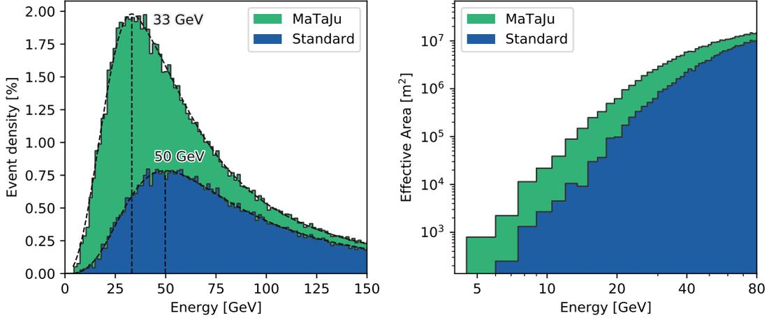
**Figure 4.6:** Comparison of the analysis threshold and effective area for the standard and MaTaju cleanings, computed for a gamma-ray source with a power-law spectrum and a spectral index  $\Gamma = 2.6$ , after the stereo reconstruction.
