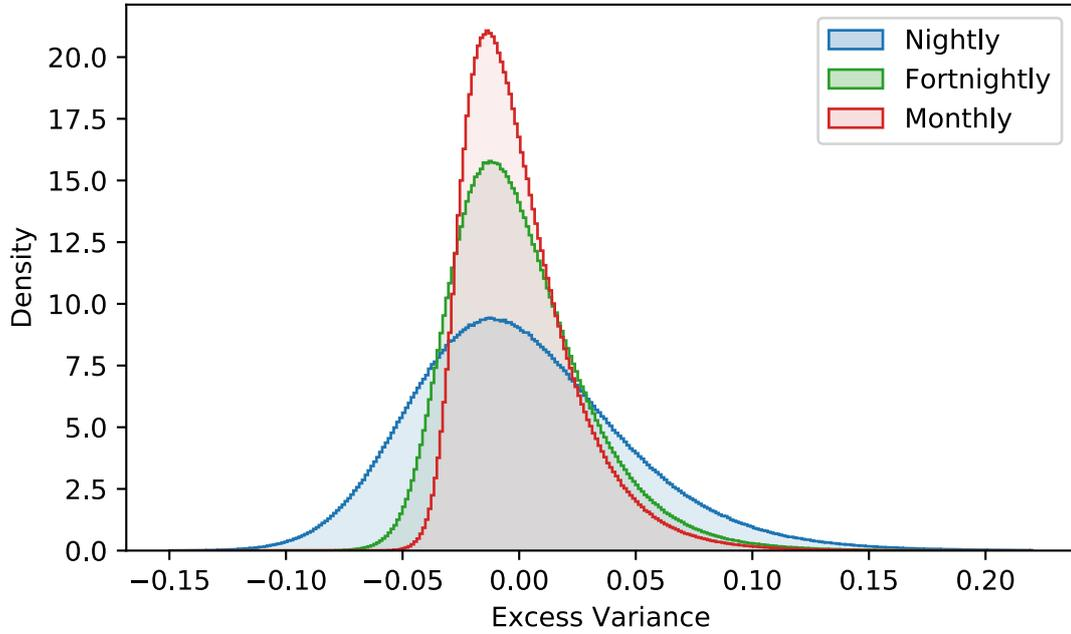
**Figure 5.13:** Excess variance distributions from Monte-Carlo simulations of  $N = 10^7$  lightcurves with realistic pulsar fluxes and observation time distributions. Stable pulsar emission ( $\Delta = 0$ ) was assumed.
