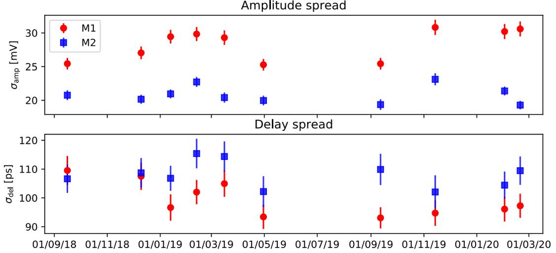
**Figure 3.5:** Spread of the amplitude and delay distribution in time (as standard deviation) for both the M1 and M2 Sum-Trigger-II. A re-calibration was done on the 30/04/2019, following the replacement of a defective clip-board in the M1 trigger.
