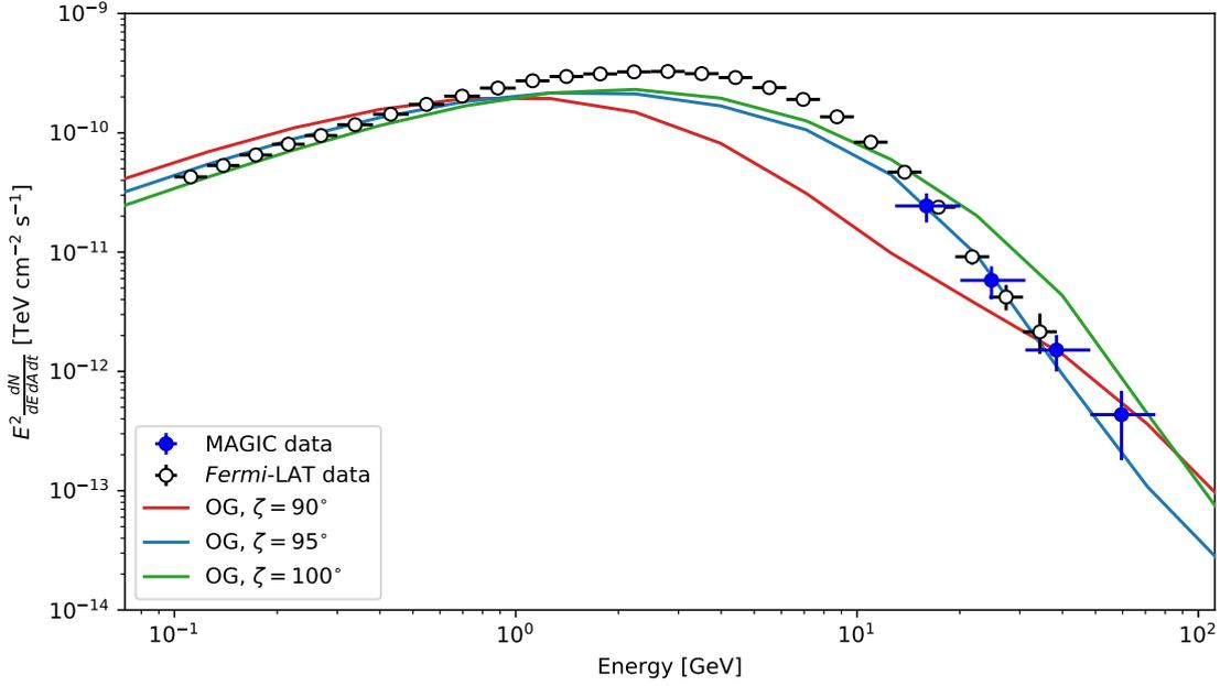
**Figure 6.12:** Set of theoretical predictions for the Geminga P2 emission, simulated according to the Outer Gap model. Curves shown are for a magnetic inclination  $\alpha = 30^\circ$ , a magnetic moment  $\mu = 1.4\mu_d$  and three different viewing angles  $\zeta$ . Simulations were produced by Dr. K. Hirotani. Curves are not fit to the data.
