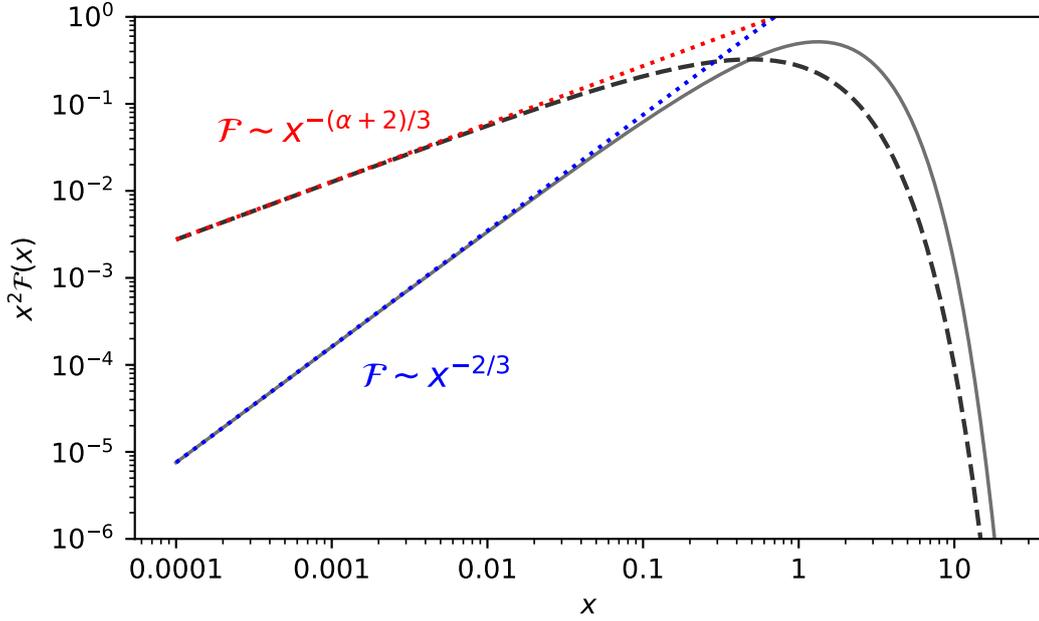
**Figure 1.4:** Sample curvature radiation spectra. Solid line: spectral energy distribution of a mono-energetic population of particles, as a function of  $x = E/E_c$  (cfr. Equation 1.8). Dashed line: same with a particle population whose energy is distributed as a power-law with spectral index  $\alpha = 2$ . Curves are normalized so that the total emitted energy is the same in both cases.
