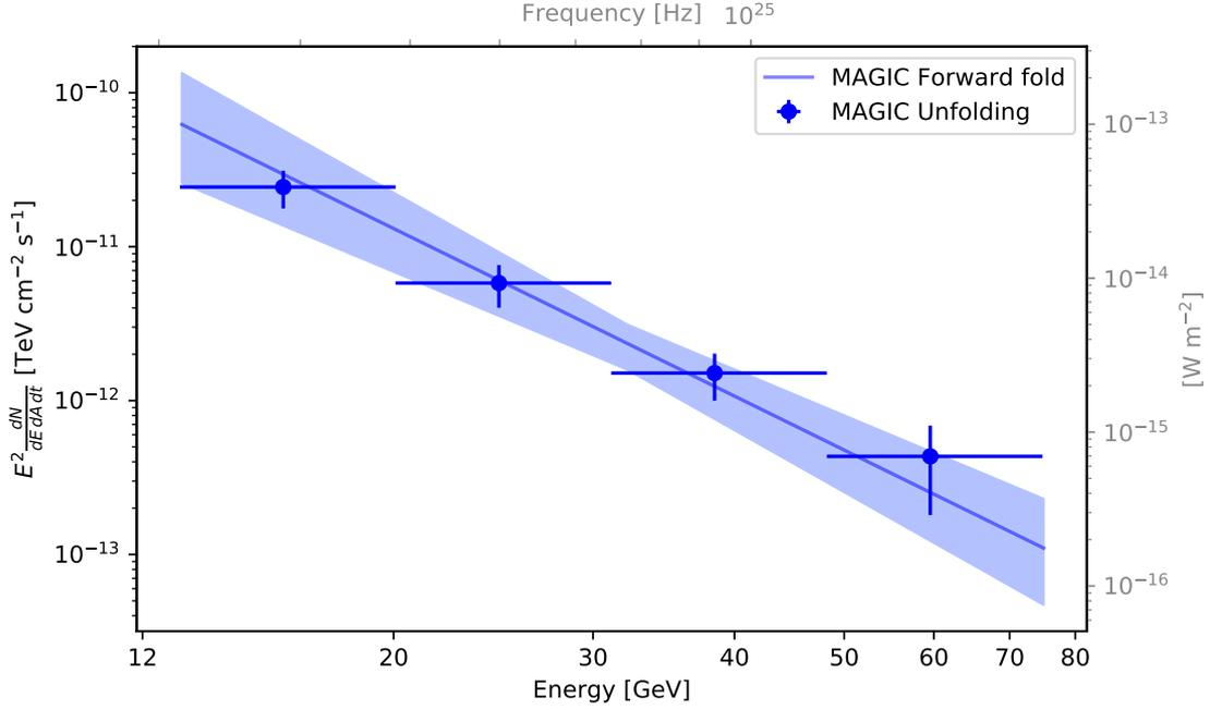
**Figure 6.6:** MAGIC spectrum of Geminga. Spectral points were produced with an unfolding procedure (Tikhonov regularization). The power-law parameters (solid line) were obtained instead with the forward folding method. Its error band gives the  $1\sigma$  confidence interval. The power-law parameters are listed in Table 6.2, while the values of the spectral points are given in Table 6.3.
