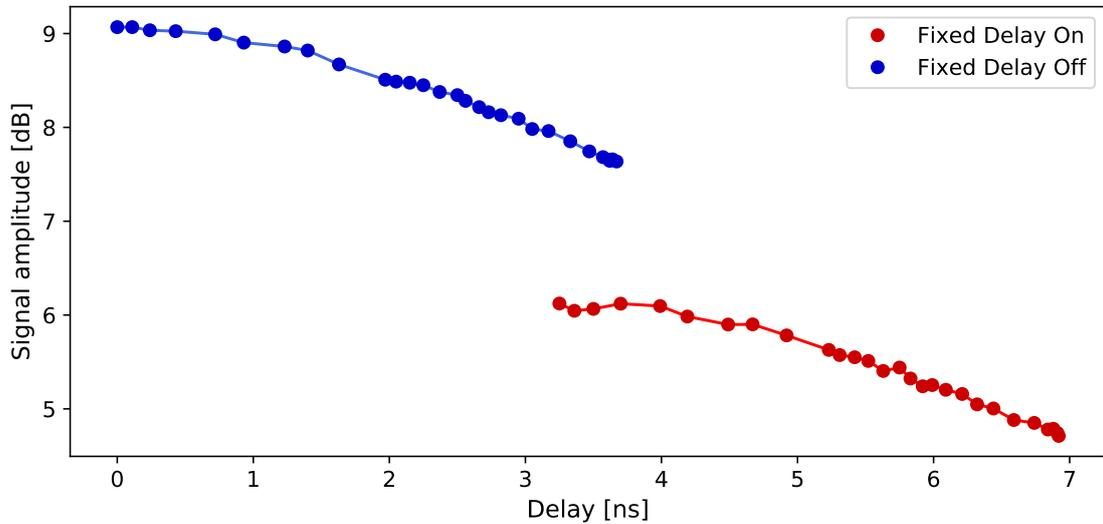
**Figure 3.3:** Delay-induced attenuation in the signals on the Sum-Trigger-II clip-boards. The red series of points corresponds to signals for which the additional fixed delay of  $\sim 3$  ns has been enabled. These values are used to build a look-up table and adjust the previously determined signal attenuation values during and after a new best delay scan.
