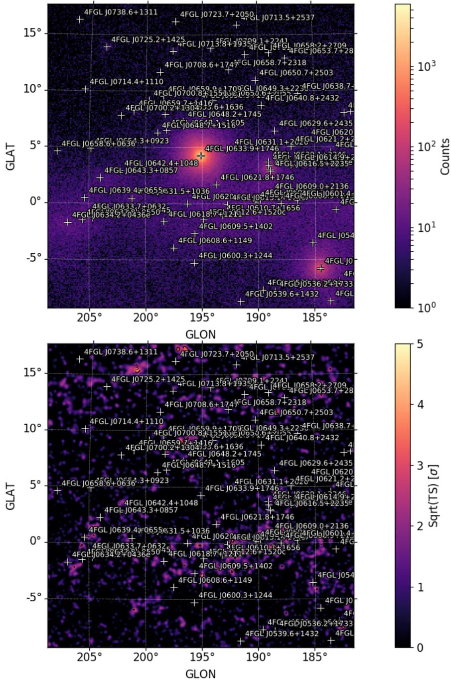
**Figure 6.2:** Upper plot: map of the counts in the *Fermi*–LAT region of interest of 30 deg around Geminga (bright spot in the center). Lower plot: significance of the residuals of the fit, as square root of the TS value. No significant residual emission is found, indicating a good fit. The bright spot in the lower right part of the count map is the Crab pulsar.
