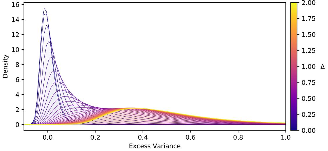
**Figure 5.15:** Excess variance  $\sigma_{NXS}^2$  distributions for toy Monte-Carlo simulations of fortnightly lightcurves. A constant pulsar flux, with the addition of a red noise is assumed:  $F(t) = F_0(1 + \Delta\mathcal{R}(t))$ . The curve for  $\Delta = 0$  is equivalent to the one in Figure 5.13.
