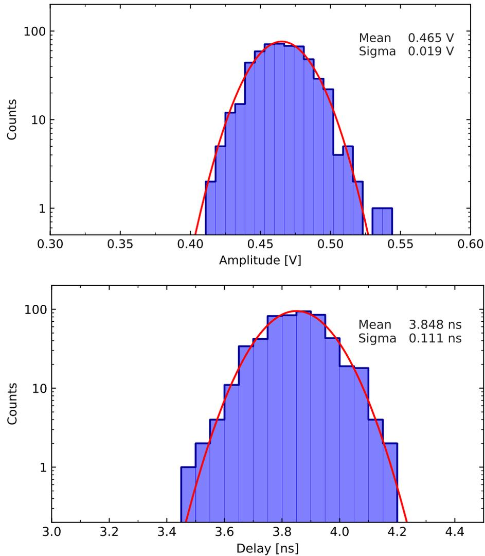
**Figure 3.4:** Distributions of the pixel amplitude and delay for MAGIC-II. These plots were obtained from a calibration test ran on February 20, 2020. The distribution are well approximated by normal ones (red line fit) with standard deviation  $\sigma_{\text{amp}} = 19 \text{ mV}$  and  $\sigma_{\text{del}} = 111 \text{ ps}$ , respectively. These are well within the operation limits for the Sum-Trigger-II.
