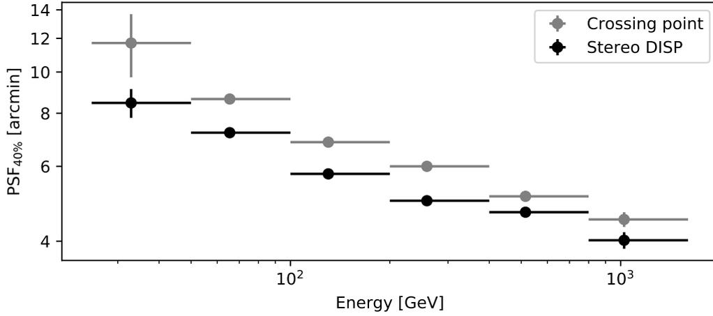
**Figure 4.16:** Energy evolution of the MAGIC point spread function for gamma rays, defined as the  $\sigma$  of a bi-dimensional Gaussian ( $\sim 40\%$  containment radius). The values were determined with Crab Nebula observations. The errors bars of the two series of points are highly correlated.
