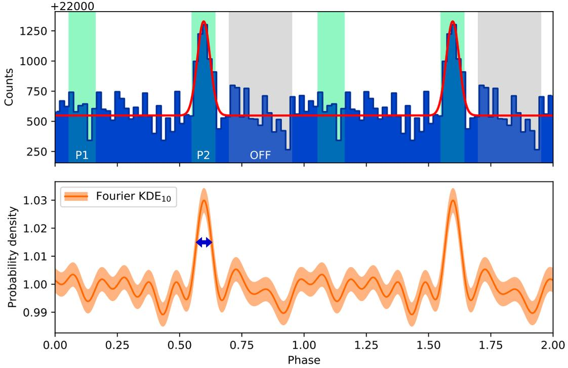
**Figure 6.5:** **Top:** MAGIC Geminga phaseogram of Figure 6.3 with the fitted cyclic Gaussian function. **Bottom:** probability density function for the phase, estimated with a Fourier kernel with  $n = 10$  harmonics, with a 68% error band.
