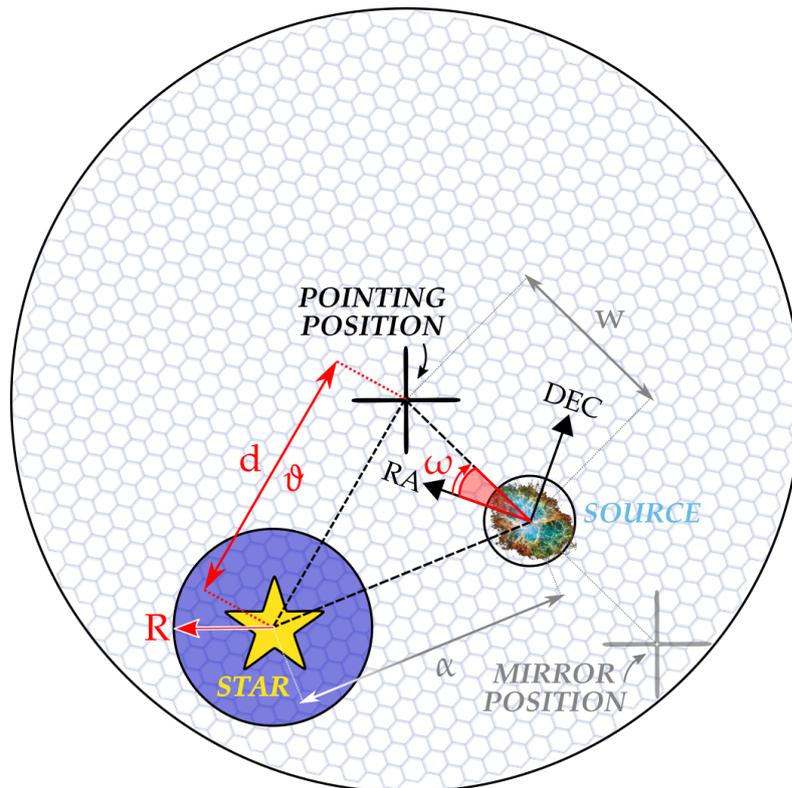
**Figure 4.13:** Sketch of the variables listed in Table 4.2, highlighted in red. The drawing shows also the wobble depth  $w$ , the star-source distance  $\alpha$  and the mirror wobble position. The RA/DEC axes do not coincide, in general, with the camera axes, and rotate during the observations.
