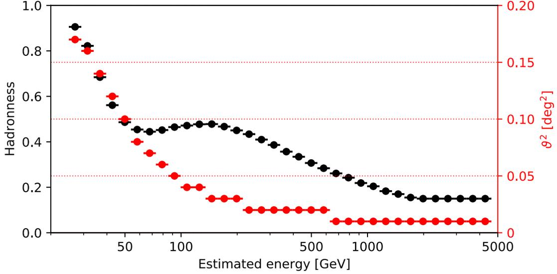
**Figure 4.19:** Energy dependent hadronness (black) and  $\theta^2$  (red) cuts, optimized for gamma-ray efficiencies of 90% and 75%, respectively. The loose  $\theta \geq 0.3$  deg cut at energies below 50 GeV affects the feasibility of the standard background estimation methods.
