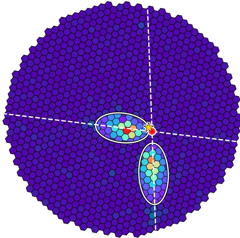
**Figure 4.8:** Stereo reconstruction. The Hillas parametrizations of an event in the two MAGIC cameras are used to determine the primary particle incoming direction (red dot). The star highlights the real incoming direction of this 430 GeV simulated gamma event.
