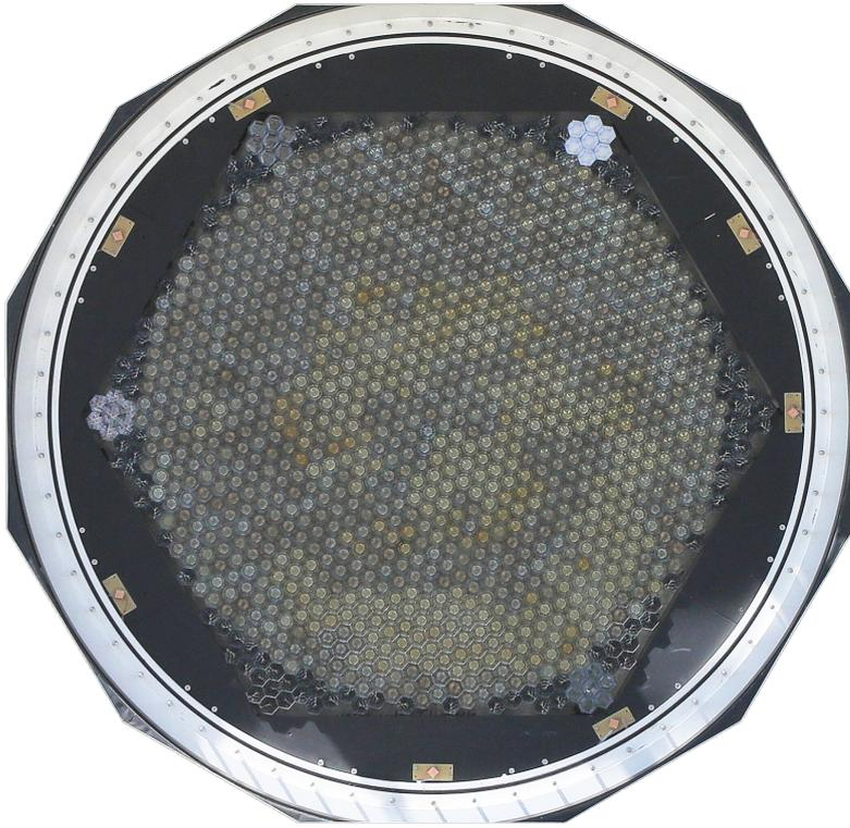
**Figure 2.8:** Close-up view of the MAGIC-I camera, without the sealed protective window. The Winston cones at the top of each photo-multiplier tube are visible. These are arranged in an hexagonal grid of 1039 pixels. Four experimental silicon photo-multiplier clusters are placed at the corners of the main sensor. The representation of a sample Cherenkov event detected by such camera is presented in Figure 4.3. *Courtesy of A. Hahn (A. Hahn / MPI).*
