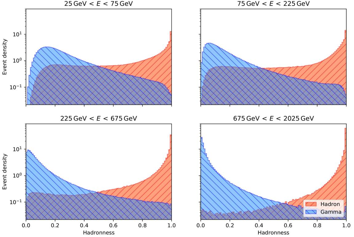
**Figure 4.14:** Comparison of the normalized hadronness distributions for gamma-rays (blue, simulation) and cosmic-rays (red, real events). The separation power degrades at lower energies. Gamma-rays were simulated with a spectral index  $\Gamma = 1.6$ , whereas the hadrons follow the cosmic-ray spectrum with  $\Gamma \simeq 2.7$ .
