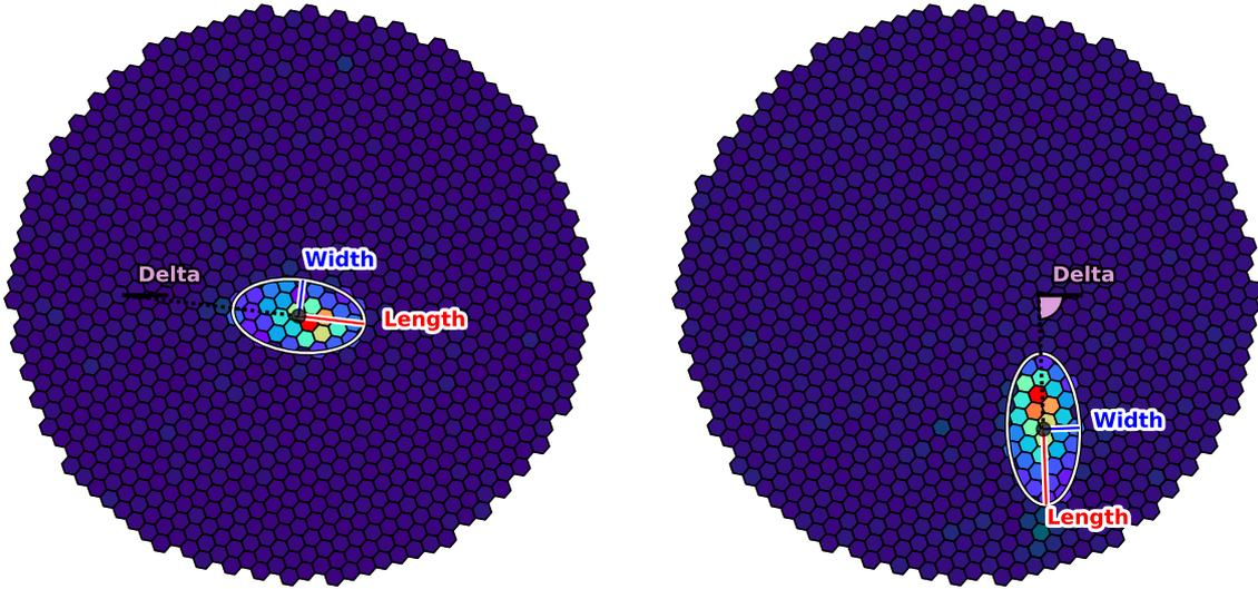
**Figure 4.7:** Hillas parametrization of an event in both MAGIC cameras, with some key parameters. The shape ones define an ellipse, drawn as the 99.7% ( $3.41\sigma$ ) containment radius of a bi-dimensional Gaussian. The darker pixels outside of the ellipses did not survive the image cleaning.
