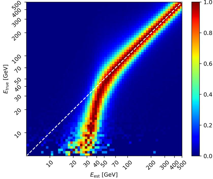
**Figure 4.17:** Energy *migration matrix* for the look-up table estimation method. The plot is normalized so that each horizontal slice (distribution of  $E_{\text{est}}$  for a given  $E_{\text{true}}$ ) peaks at 1. The fuzziness at  $E_{\text{true}} < 10$  GeV is caused by the reduction of the Monte-Carlo statistics. Events with a zenith distance  $\zeta < 30$  deg were used to produce the plot.
