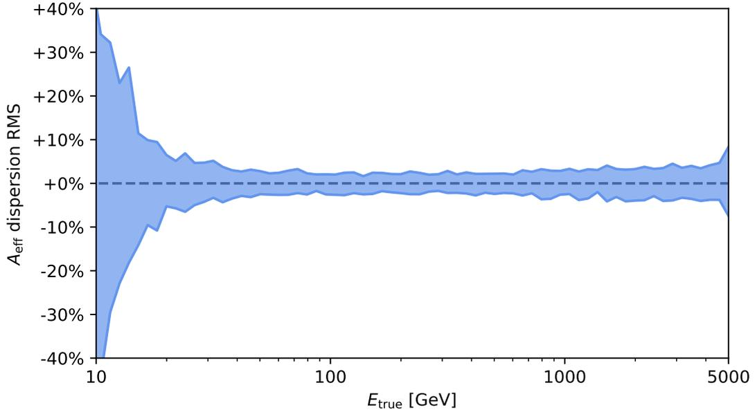
**Figure 4.25:** Relative dispersion of the effective area caused by a low-statistic Monte-Carlo ( $2.5 \cdot 10^6$  events, the standard size in MAGIC). The colored band represents the  $1\sigma$  region for the fluctuations around the average. Obtained by bootstrapping samples from a larger Monte-Carlo set ( $1.35 \cdot 10^8$  events, production codes 11+12+13+14 in Table 4.4).
