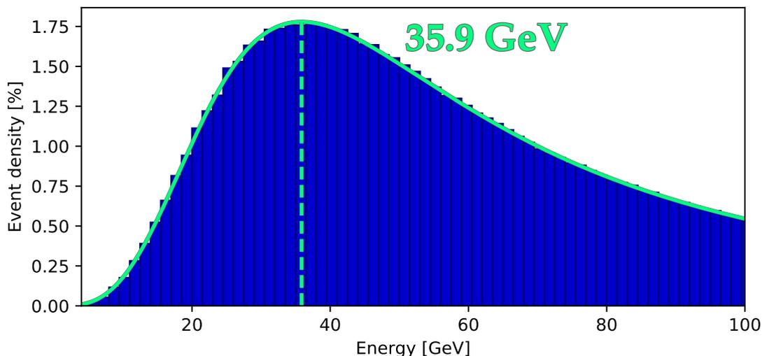
**Figure 4.23:** Normalized true energy distribution for Monte-Carlo events analyzed with the pipeline presented in this chapter, for a power-law spectrum with spectral index  $\Gamma = 2.6$ . An energy threshold of  $E_{\text{thr}} = 36$  GeV is achieved for this spectral shape.
