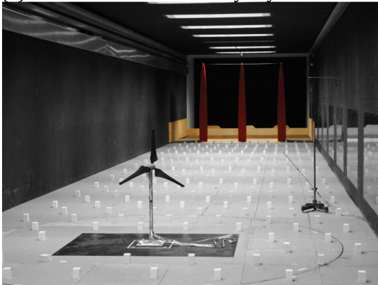
Figure 5.1: View of the Model Wind Turbine located within (a) the smooth boundary layer and (b) the rough boundary layer configuration of the wind tunnel.
