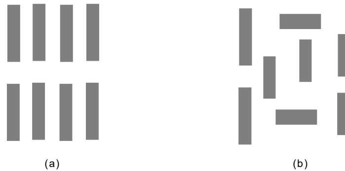
Figure 46: Sketch of urban design with examples of horizontal distribution of buildings. Note: (a) homogeneous grid, and (b) heterogeneous one. No scale. Source: own author.
