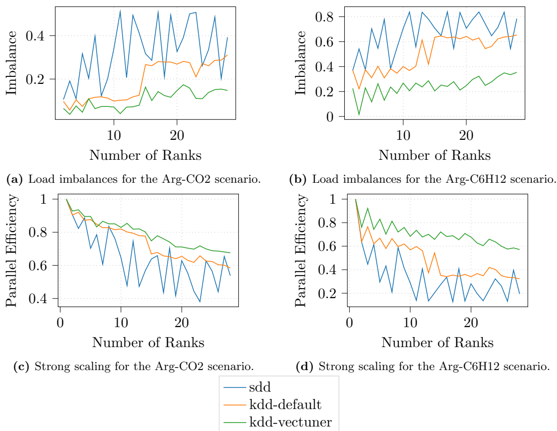
Figure 4.13: Load imbalances and strong scaling for the Arg-CO2 and Arg-C6H12 scenarios on one node of CoolMUC2 for the kdd using the new (vectorization tuner) and old load estimator. As comparison results using the standard Cartesian domain decomposition (sdd) are given.
