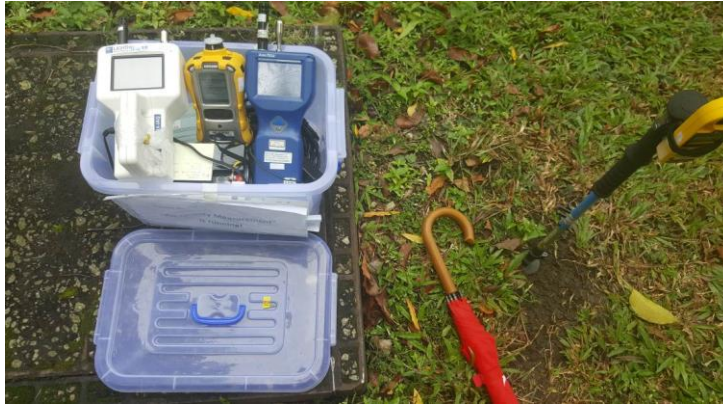
Figure 6-18: Location (4), box 1: air quality monitoring instrument (wind tracker, particle counters, and multi-gas detector)
