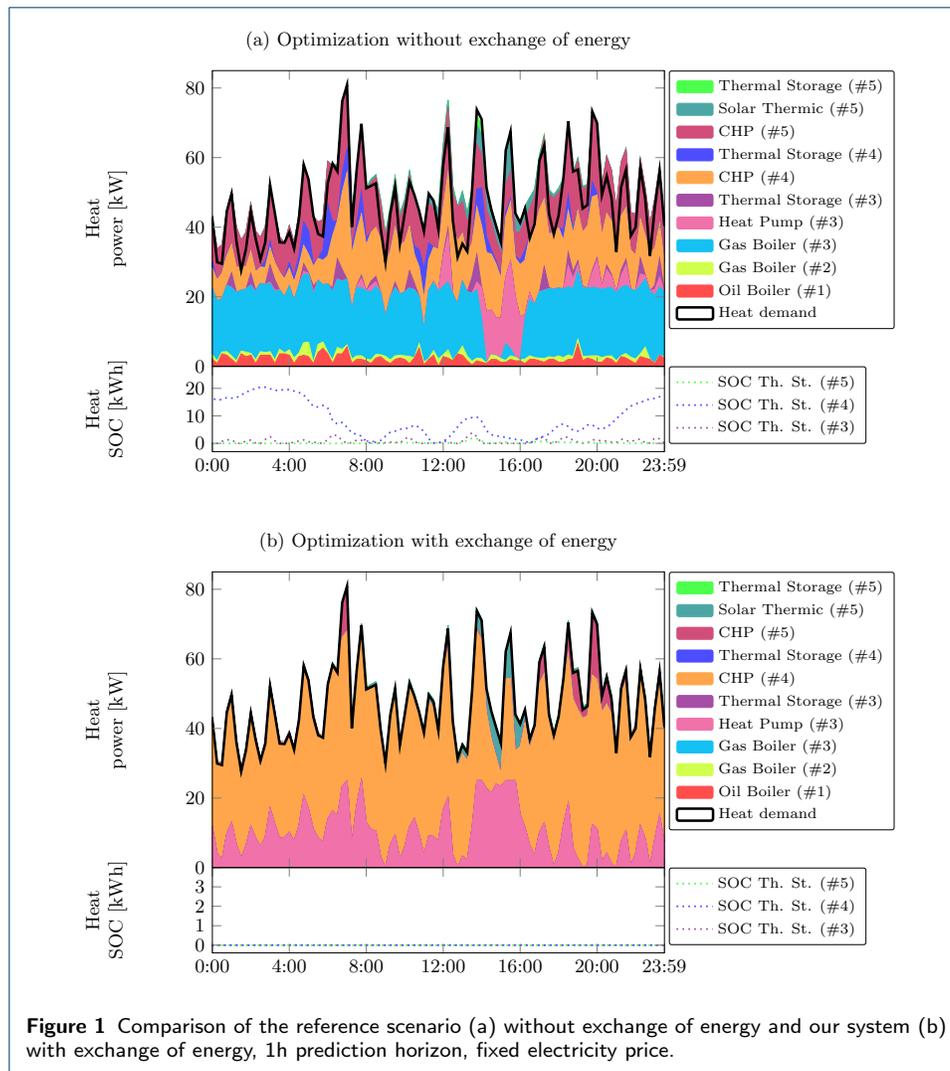
**Figure 1** Comparison of the reference scenario (a) without exchange of energy and our system (b) with exchange of energy, 1h prediction horizon, fixed electricity price.
