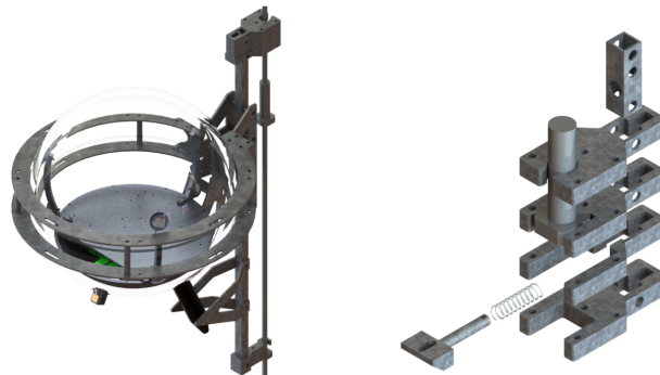
Figure 4.8: Technical drawing of the external mounting for a glass sphere module of STRAWb. Picture courtesy of Christian Spannfellner.
