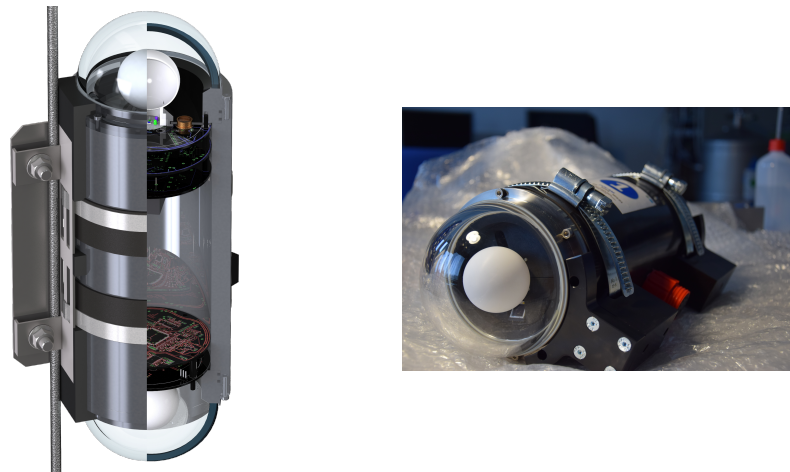
Figure 3.11: Left: Sketch of the POCAM housing: a titanium cylinder with BK-7 glass hemispheres on both ends. Right: Picture of the first complete POCAM before shipment.
