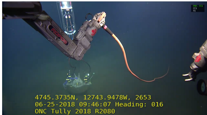
Figure 3.9: The ROV arm holding the cable during the connection operations of the yellow string.
