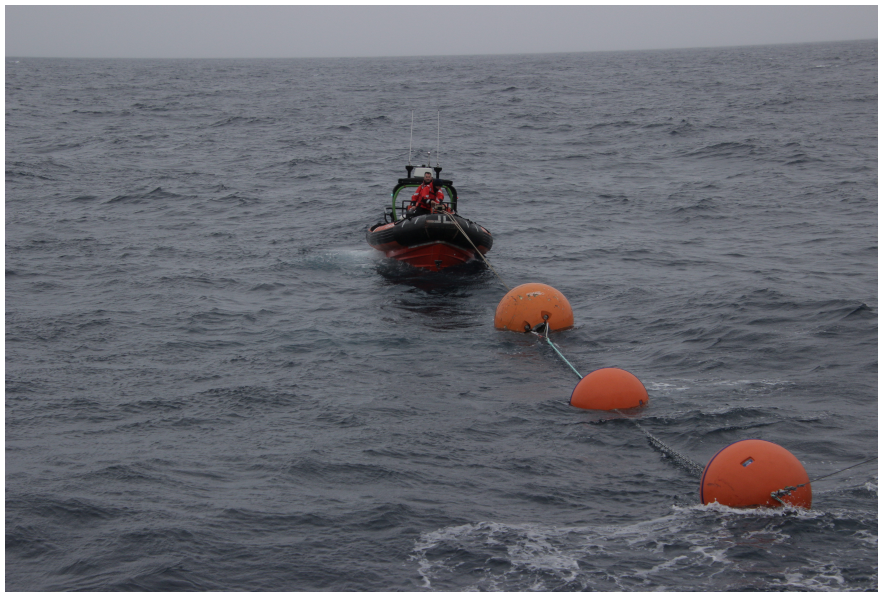
Figure 4.9: First phase of deployment operations: the buoys are dragged far from the ship to have the string well stretched on the sea surface. Credits to Will Glatt and Tammy Gomez (ONC).
