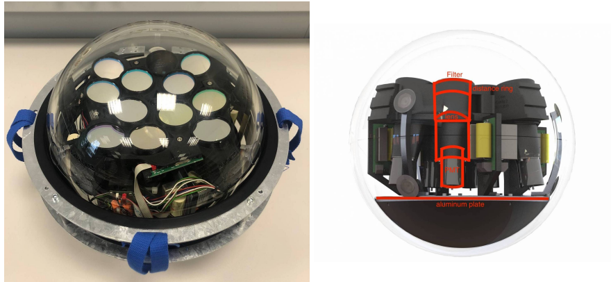
Figure 4.16: Left: Frontal picture of one of the two PMT spectrometer modules before shipping them to Canada. Right: Technical drawing of the internal 3D support structure designed by Kilian Holzappel.
