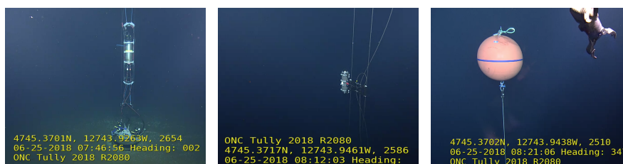
Figure 3.8: Pictures of STRAW from the ROV visual inspection right after the deployment.
