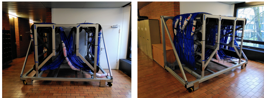
Figure 4.6: Picture of the tray with all 10 VEOCs spooled on it. Pictures courtesy of Christian Spanneller [6]
