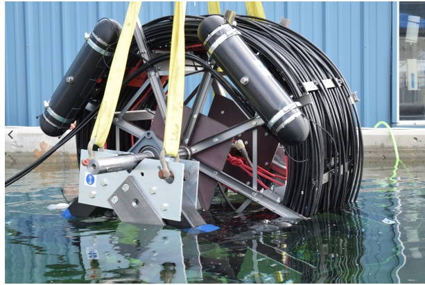
Figure 3.17: One string entering the pool for final underwater functional tests at MTC some days before the deployment.
