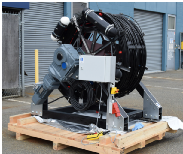
Figure 3.5: One of the two spooling systems once arrived at Marine Technology Center in Victoria, Canada: all the modules are covered for light protection and secured to the winch.
