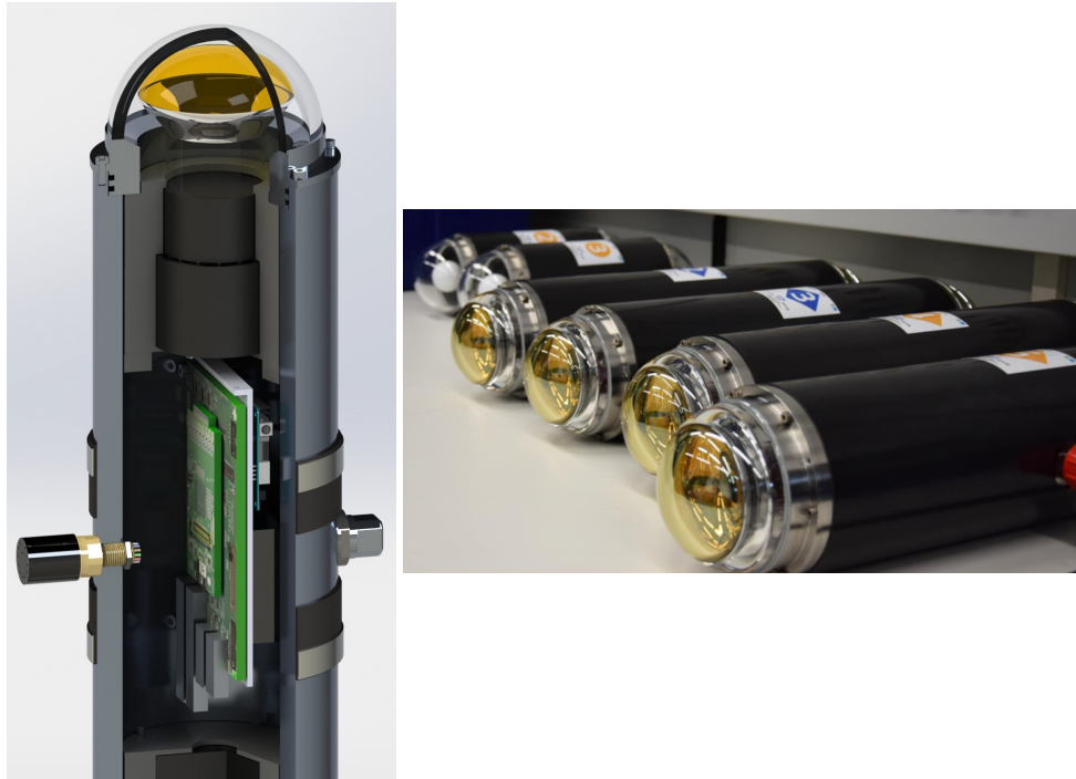
Figure 3.15: Left: Schematic design of the sDOM. Right: Picture of the sDOMs and POCAMs ready for the shipment to Canada. Picture courtesy of Felix Henningsen [51].
