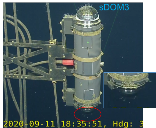
Figure 5.32: Picture of the sDOM3 taken during the inspection of STRAW moorings in September 2020: the presence of both biofouling and sediment on the glass hemispheres is visible.
