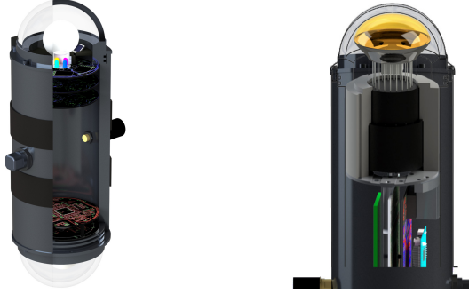
Figure 3.1: Left: The POCAM housing. Titanium cylinder with BK-7 glass hemispheres on either ends allowing isotropic light emission. Right: sDOM (POCAM-like) housing with PMT and electronics.
