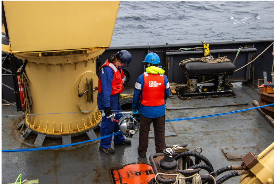
Figure 4.10: Picture taken during deployment operation: the crew members are connecting the module to the steel cable. Credits to Will Glatt and Tammy Gomez (ONC).
