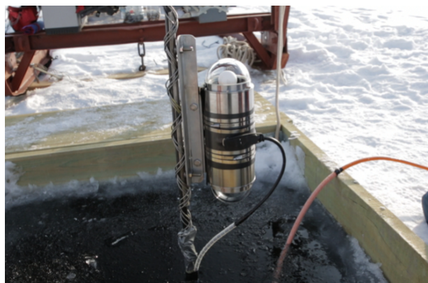
Figure 3.10: Deployment of one POCAM module into GVD detector - lake Baikal, southern Siberia. Picture courtesy of Felix Henningsen.
