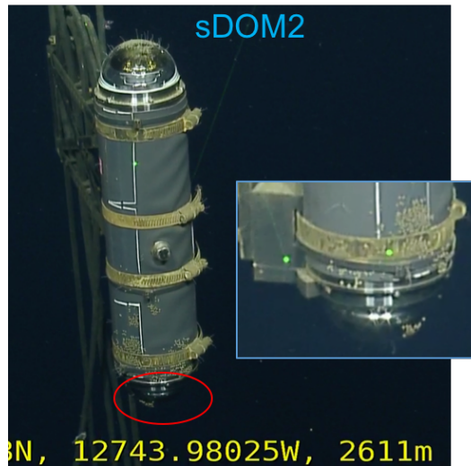
Figure 5.31: Picture of the sDOM2 taken during the inspection of STRAW moorings in September 2020: the presence of both biofouling and sediment on the glass hemispheres is visible.
