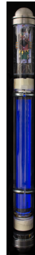
Figure 4.18: Picture of the WOM: the detector is illuminated by UV light to show the fluorescence of the wavelength shifter. Courtesy of JGU Mainz group.
