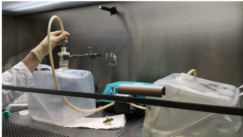
Figure 26: Filtration of river water by MAF-DEAE under flow hood.
