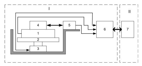
**Figure 1.** Block diagram of a dynamic laser goniometer; 1—ring laser, 2—rotary platform, 3—drive, 4—rotor, 5—stator of the angle converter, 6—electronics unit, 7—computer.
