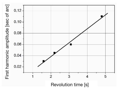
Figure 4. The dependence of the amplitude of the first harmonic on the revolution time.
