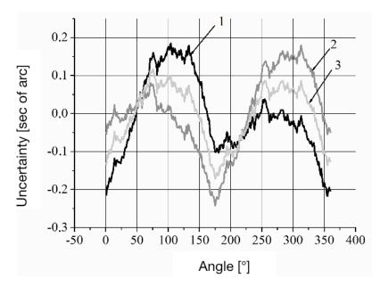
**Figure 3.** Illustration of the systematic error of the LDG: 1—RL CCW rotation; 2—RL CW rotation; 3—systematic error of the optical encoder.
