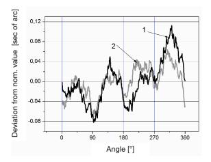
**Figure 6.** The results of the RON-905 calibration with rotation of the rotor in CW (2) and CCW direction (1).
