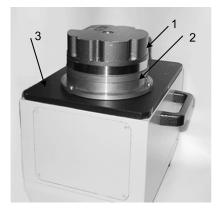
**Figure 5.** Installation of the LDG for the calibration of optical encoders; 1—RON-905; 2—adjustment ring; 3—LDG.
