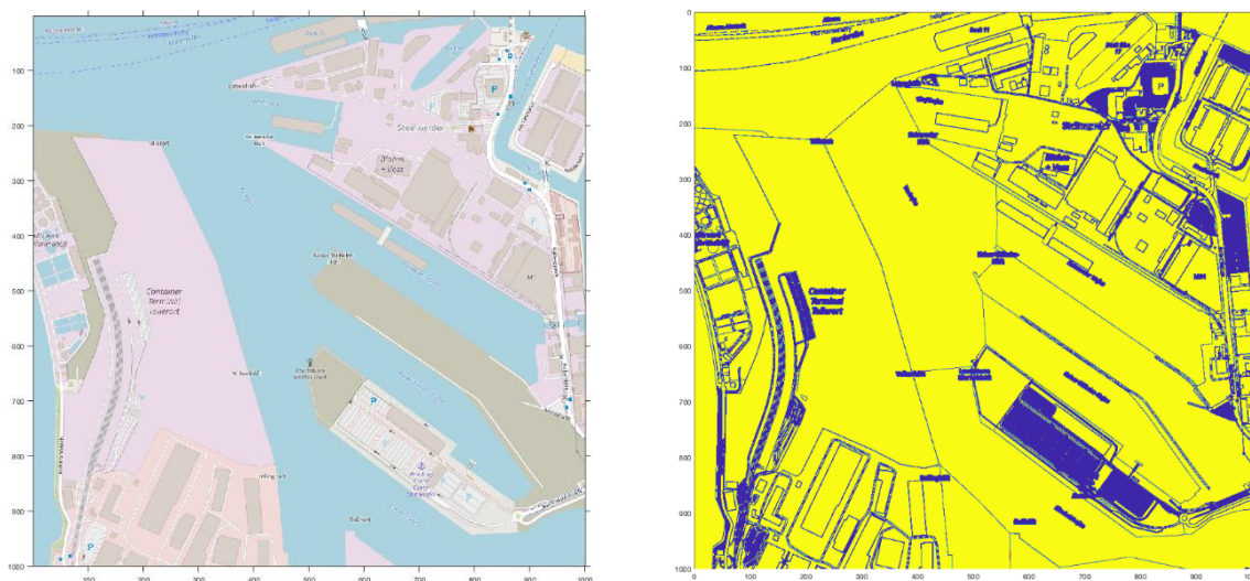
Figure 7-7. Left: OSM image part of Hamburg harbour. Right: Basic MapScan result, detection rate 83.99 %.
