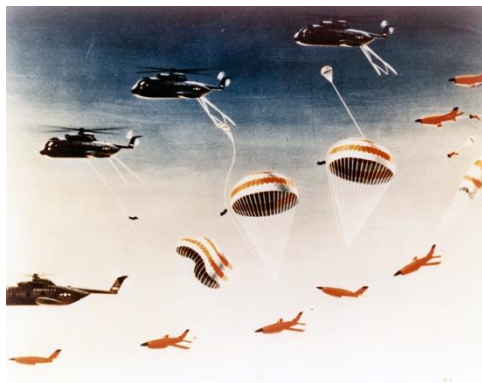
Figure 2-10. AQM-34 - Medium Air Retrieval System illustration, year unknown 10 .
