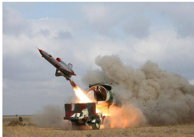
Figure 2-12. Rocket-assisted launch of Tu-143, 2016 12 .
