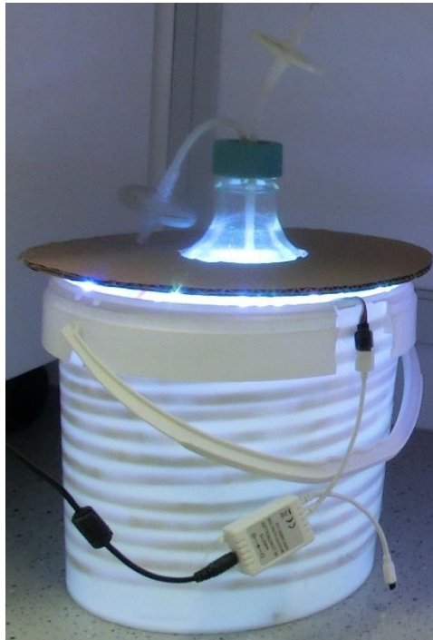
Figure 3.2. 4.5 L cylinder cultivation system. It allowed to cultivate both strains in order produce EPS for both Porphyridum EPSs rheological characterization.
