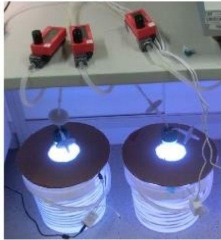
Fig. S 1. 5 L Cultivation system used in this investigation. The system was run at room temperature (RT), with a white fluorescence LED 10 m (SimpLED, 300 LED, Paulmann). The air inlet was fixed at 2000 \text{ mL min}^{-1} with a flowmeter (Red-y for gas flow, Switzerland), in 4500 mL of culture volume. The air deliver system was assembled using 0.3–0.5 mm silicon tubing, with one Y polypropylene connection (Bürkle), two T polypropylene connections (Bürkle), and two 0.2 \mu\text{m} PTFE filters Midisart 2000 (Sartorius Stedim).
