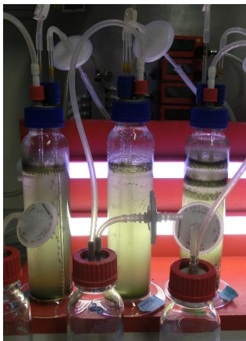
Figure 3.1 0.5 L cylinder cultivation system. It allowed to cultivate both strains in order to evaluate their growth behavior, nutrient uptake and EPS characterization tests.
