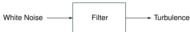
Figure 2.9.: Illustration of atmospheric turbulence simulation using a shaping filter. Figure taken from Ref. [258].
