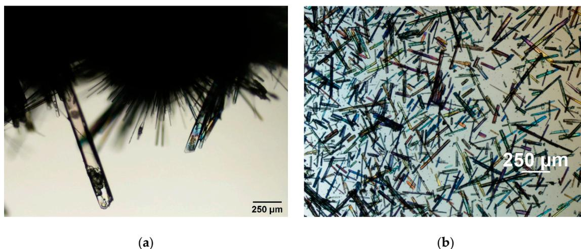
**Figure 2.**  $\gamma$ -NADA crystals obtained with cooling crystallization ( $50\text{ }^\circ\text{C}$ – $20\text{ }^\circ\text{C}$ ) in  $\text{H}_2\text{O}$ . (a)  $\gamma$ -NADA crystal cluster after crystallization in 2 mL reaction tube in  $\text{H}_2\text{O}$  with 300 rpm shaking. (b) Single crystals after crystallization in a small scale reactor with 150 rpm stirring and 10 mL volume.
