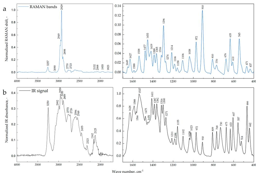
**Figure 5.** Raman (a) and IR spectra (b) of crystalline  $\gamma$ -acetyl-L-2,4-diaminobutyric acid, obtained from cooling crystallization in  $\text{H}_2\text{O}$ . The signal was normalized to the most pronounced peak, namely at  $2929\text{ cm}^{-1}$  and  $1537\text{ cm}^{-1}$  for Raman and IR spectroscopy, respectively. For the detailed assignment of the bands, see Table S9.
