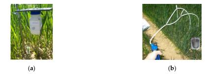
**Figure 2.** Passive-flux-collector from a square bottle with a modified acid trap for  $NH_3$  (**a**) and Dräger-Tuber method (DTM) with Teflon tubes for hand pumping (**b**).
