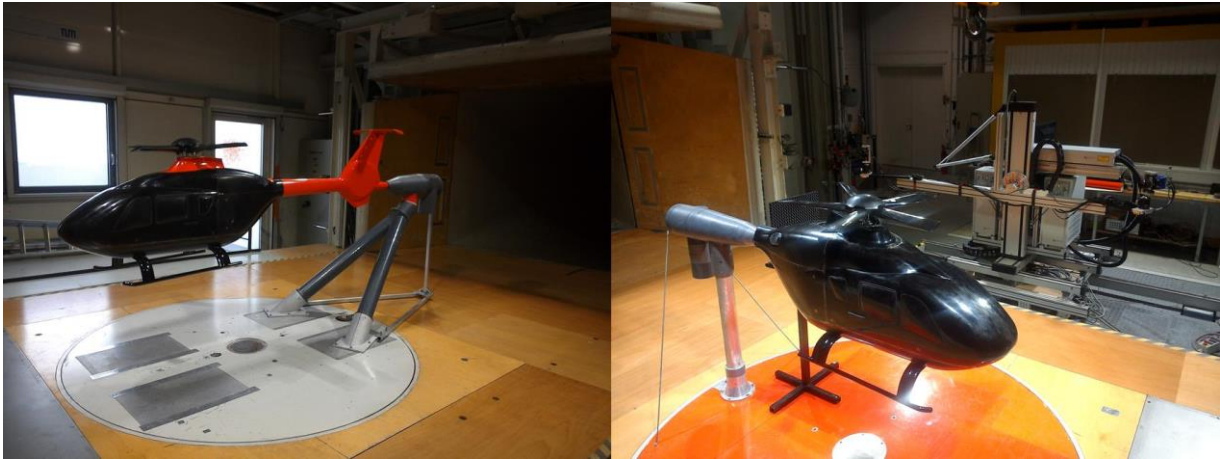
Figure 108: Wind tunnel configurations. The full model (left) and the model without tail sting-mounted (right) in the wind tunnel is presented.
