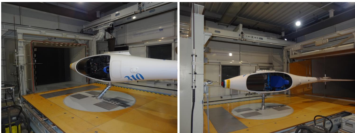
Figure 97: Test configuration mounted in the test section of the wind tunnel. View in direction of the nozzle (left) and in the direction of the diffuser (right) is shown. Propeller and spinner are not shown.
