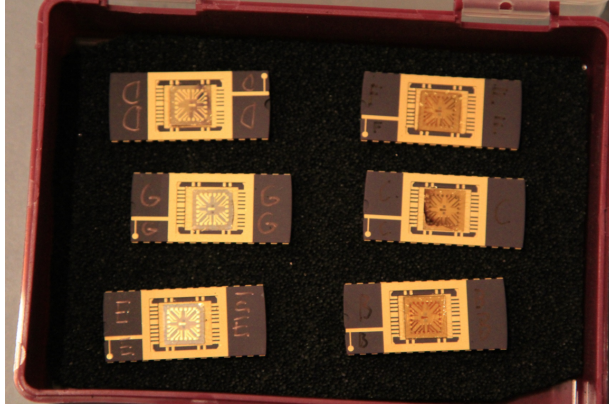
FIGURE 3.6: GaN-HEMT devices produced as part of this thesis inside a transport box after completion of the bonding procedure.
