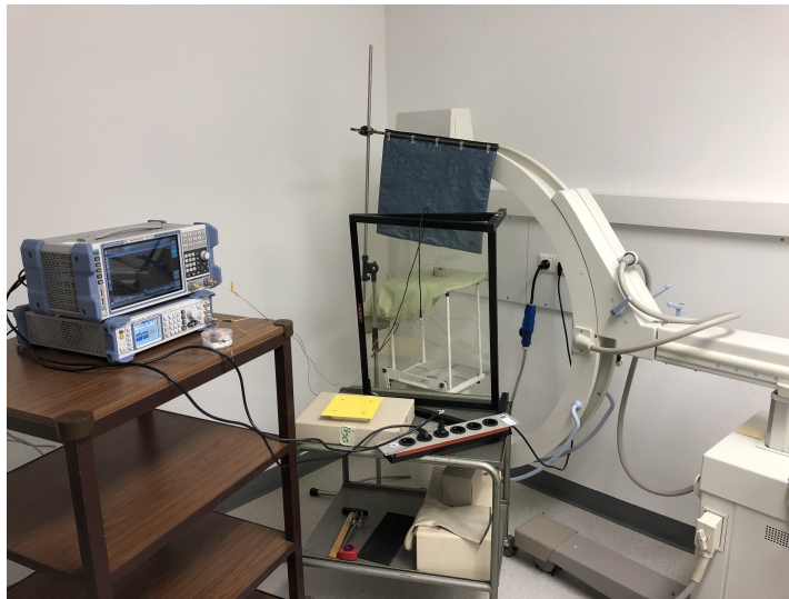
FIGURE 3.16: Side view of the C-arm fluoroscopy X-ray system used in this thesis, with the measurement equipment on the left side and the radiation protection equipment in front of the sample.
