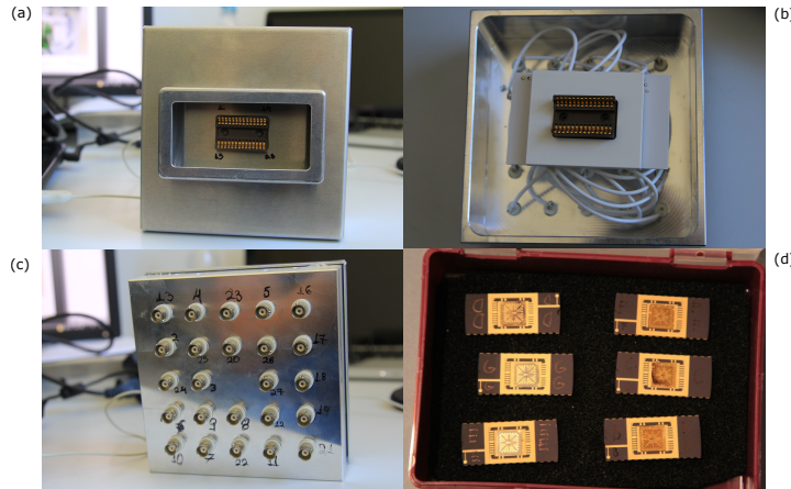
FIGURE 3.10: (a) Front view of measurement box with the socket for the chip carrier. (b) Inside view of the measurement box with the BNC cables soldered to the electric board. (c) Rear view of the measurement box with the BNC connectors corresponding to the individual device contacts. (d) Lead chip carriers with the bonded AlGa N /Ga N -HEMT devices.
