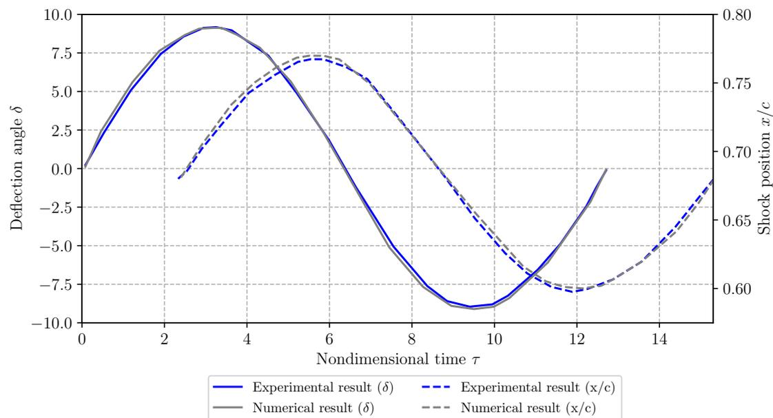
**Figure 4.** Comparison of numerical and experimental results in terms of varying aileron angle and shock position with time (NACA65<sub>1</sub>213 airfoil,  $Ma_\infty = 0.8$ ,  $Re = 20.7 \times 10^6$ ,  $\alpha = -1^\circ$ ,  $\delta = \pm 9^\circ$ ).
