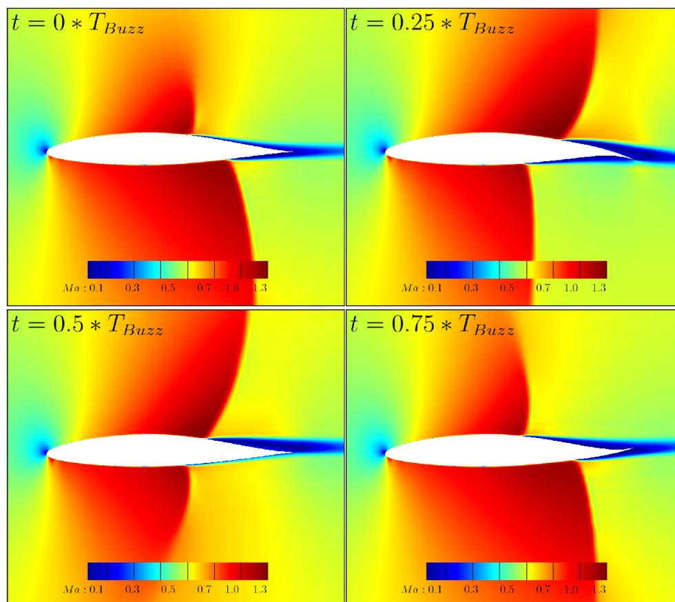
**Figure 3.** Mach number contour plots showing the buzz cycle of the NACA65<sub>1</sub>213 airfoil ( $Ma_\infty = 0.82$ ,  $Re = 20.7 \times 10^6$ ,  $\alpha = -1^\circ$ ,  $\delta = \pm 12^\circ$ ).  $T_{Buzz}$  refers to the buzz period.
