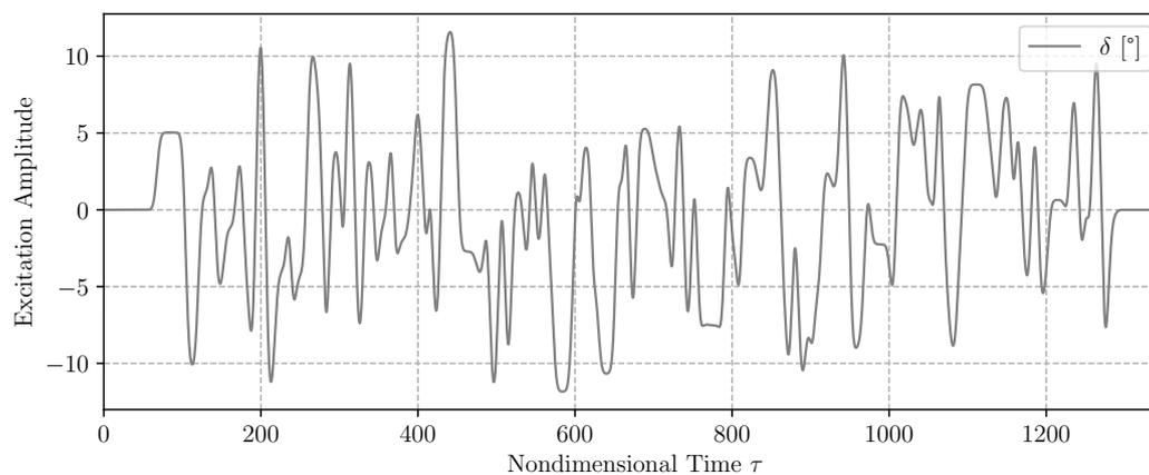
**Figure 5.** Time series of the training signal (APRBS) for the excitation of the ailerons structural degree of freedom.
