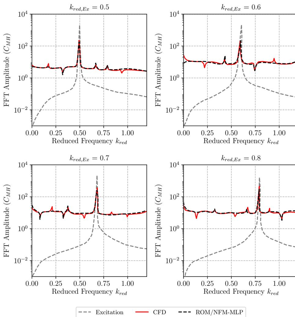
**Figure 9.** Frequency domain responses of the hinge moment coefficient resulting from harmonic aileron pitching motion with  $k_{red,Ex} = [0.5, 0.6, 0.7, 0.8]$ . The results of the NFM-MLP ROM are compared to the reference CFD solution (NACA65<sub>1</sub>213 airfoil,  $Ma_\infty = 0.82$ ,  $Re = 20.7 \times 10^6$ ,  $\alpha = -1^\circ$ ,  $\delta_{min,max} = -12/+9^\circ$ ).
