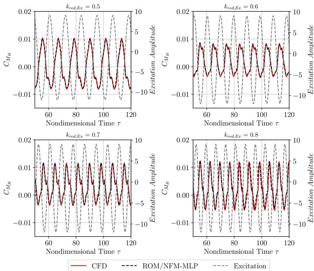
**Figure 8.** Responses of the hinge moment coefficient resulting from harmonic aileron pitching motion with  $k_{red,Ex} = [0.5, 0.6, 0.7, 0.8]$ . The results of the NFM-MLP ROM are compared to the reference CFD solution (NACA65<sub>1</sub>213 airfoil,  $Ma_\infty = 0.82$ ,  $Re = 20.7 \times 10^6$ ,  $\alpha = -1^\circ$ ,  $\delta_{min,max} = -12/+9^\circ$ ).
