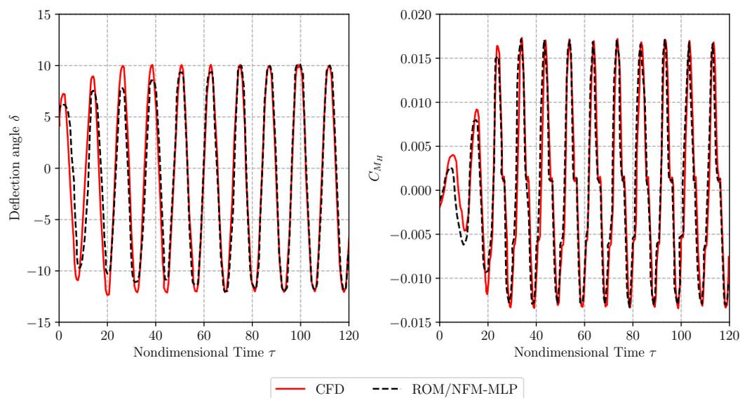
**Figure 11.** Responses of the resulting aileron deflection angle and hinge moment coefficient at a selected buzz condition (NACA65<sub>1</sub>213 airfoil,  $Ma_\infty = 0.82$ ,  $Re = 20.7 \times 10^6$ ,  $\alpha = -1^\circ$ ,  $\delta_{start} = -4^\circ$ ). The results of the NFM-MLP ROM are compared to the reference CFD solution.
