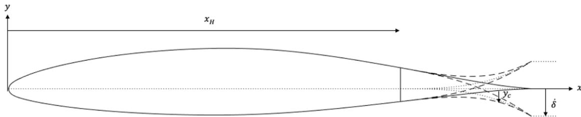
**Figure 2.** Geometry of the NACA65<sub>1</sub>213 airfoil with integrated aileron deflection.
