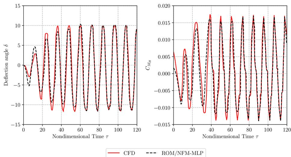
**Figure 13.** Responses of the resulting aileron deflection angle and hinge moment coefficient at a buzz condition with time decay (NACA65<sub>1</sub>213 airfoil,  $Ma_\infty = 0.8$ ,  $Re = 20.7 \times 10^6$ ,  $\alpha = -1^\circ$ ,  $\delta_{start} = 0^\circ$ ). The results of the NFM-MLP ROM are compared to the reference CFD solution.
