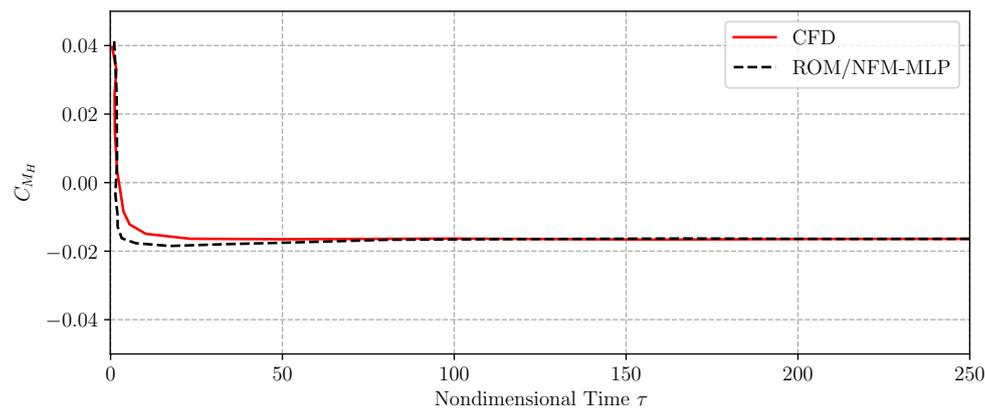
**Figure 10.** Stable aeroelastic response of the hinge moment coefficient (NACA65<sub>1</sub>213 airfoil,  $Ma_\infty = 0.8$ ,  $Re = 10^6$ ,  $\alpha = 0^\circ$ ). The result of the NFM-MLP ROM is compared to the reference CFD solution.
