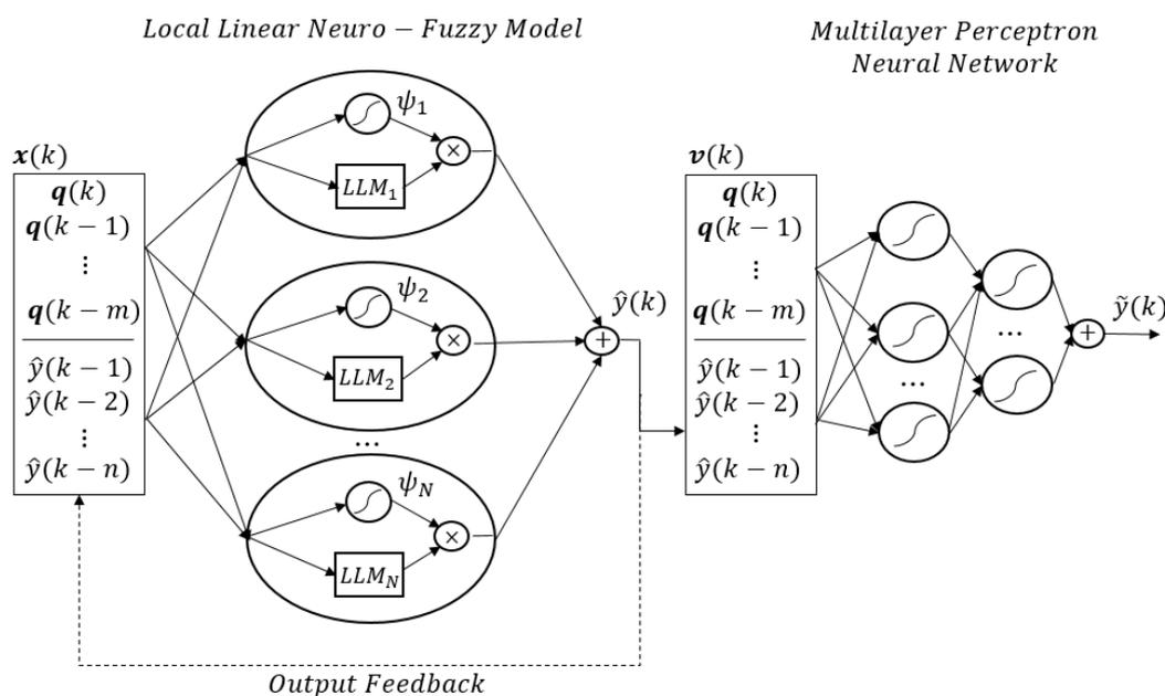
**Figure 1.** Illustration of the combined recurrent local linear neuro-fuzzy model and multilayer perceptron neural network [12].
