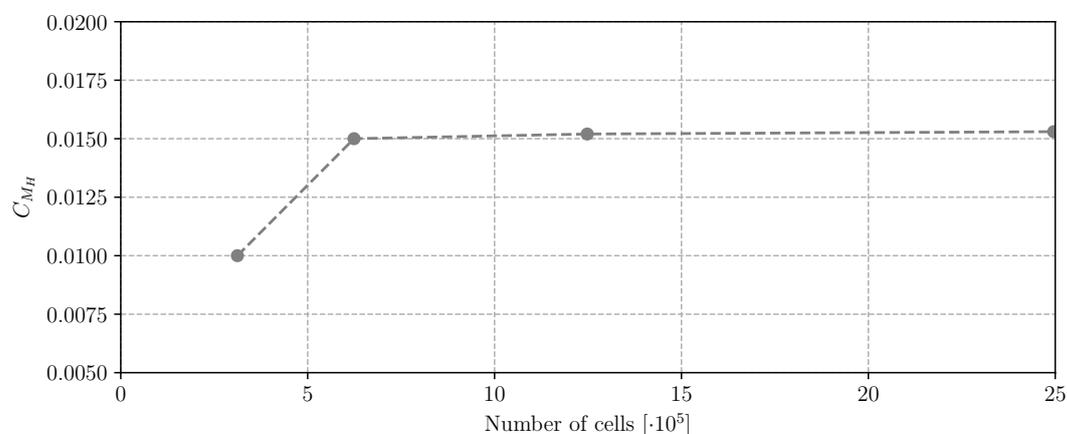
**Figure 6.** Grid convergence study with regard to the hinge moment coefficient  $C_{M_H}$  (NACA65<sub>1</sub>213 airfoil,  $Ma_\infty = 0.8$ ,  $Re = 20.7 \times 10^6$ ,  $\alpha = 0^\circ$ ,  $\delta = 0^\circ$ ).
