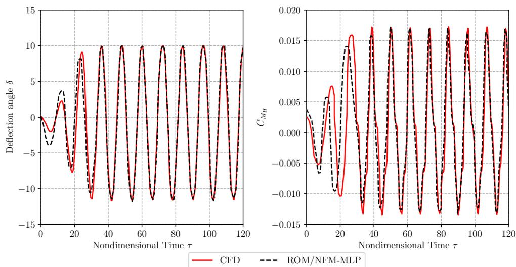
**Figure 12.** Responses of the resulting aileron deflection angle and hinge moment coefficient at a selected buzz condition (NACA65<sub>1</sub>213 airfoil,  $Ma_\infty = 0.83$ ,  $Re = 20.7 \times 10^6$ ,  $\alpha = -1^\circ$ ,  $\delta_{start} = 0^\circ$ ). The results of the NFM-MLP ROM are compared to the reference CFD solution.
