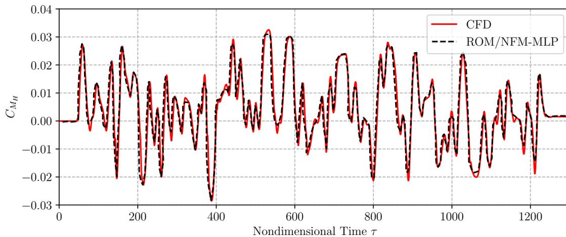
**Figure 7.** Hinge moment coefficient response caused by the APRBS excitation (NACA65<sub>1</sub>213 airfoil,  $Ma_\infty = 0.82$ ,  $Re = 20.7 \times 10^6$ ,  $\alpha = -1^\circ$ ,  $\delta = \pm 12^\circ$ ). Besides the CFD reference solution, the simulation result of the NFM-MLP ROM is shown.
