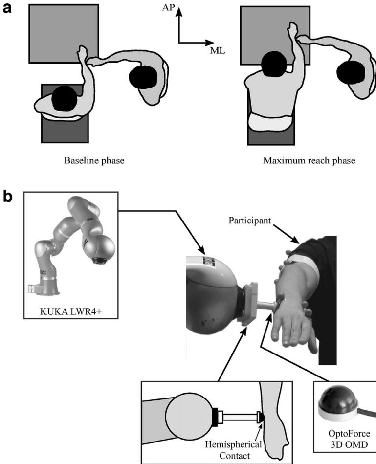
*Figure 1.* Experimental setup. (a) Execution of the maximum forward reach task with human interpersonal touch (hIPT) support. (b) Robotic IPT without mechanical coupling in hybrid force-position control.
