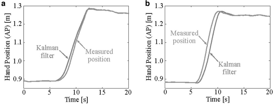
**Figure 3.** Kalman filtered hand position during maximum forward reaching (MFR). (a) Predicted and measured hand position during MFR for anticipatory robotic interpersonal touch (rIPT) in the anteroposterior (AP) direction. (b) Estimated and measured hand position during MFR for rIPT in follower mode in the AP direction.
