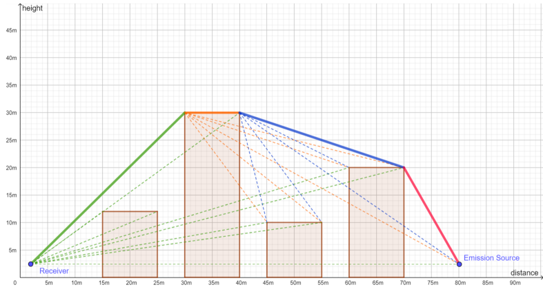
Figure 5.9: Construction of the shortest path around the obstacles, starting from the receiver on the left. After calculating the slopes to all possible edges, the edge connected with the highest slope is fixed (thick lines). The procedure is repeated starting from the last fixed edge until the emission source is reached.
