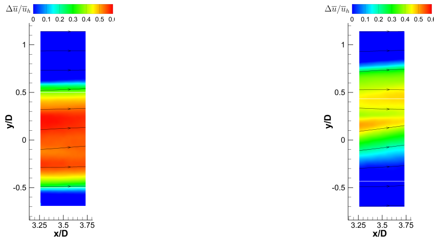
Figure 11: Contours of the normalized streamwise velocity deficit in xy planes 3.5 D downstream of the rotor for yaw angle \gamma = 0^\circ (left), and \gamma = -30^\circ (right). In-plane streamlines of the flow are also plotted. The white lines denote rotor edges.
