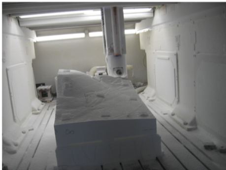
Figure 7: A complex sub-part cut by CNC machine.
