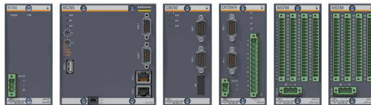
Figure 2.9: Picture of the Bachmann PLC control system.
