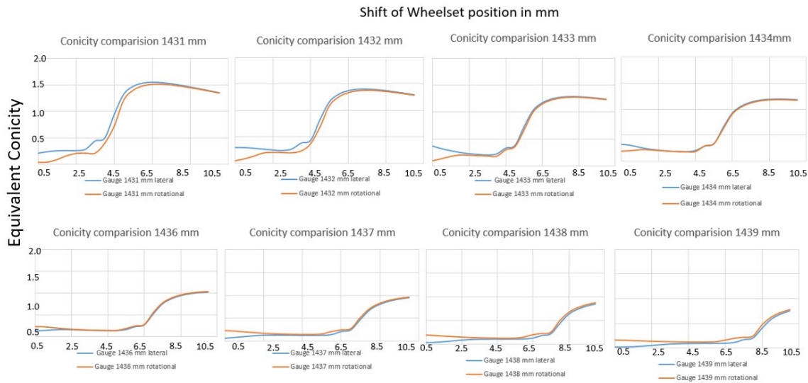
Figure 72: Equivalent conicity affected by rail rotation and rail lateral movement (standard gauge)
