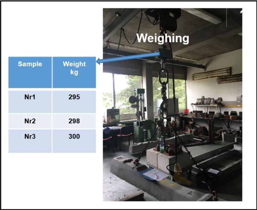
Figure 27: Weighing of sleepers
