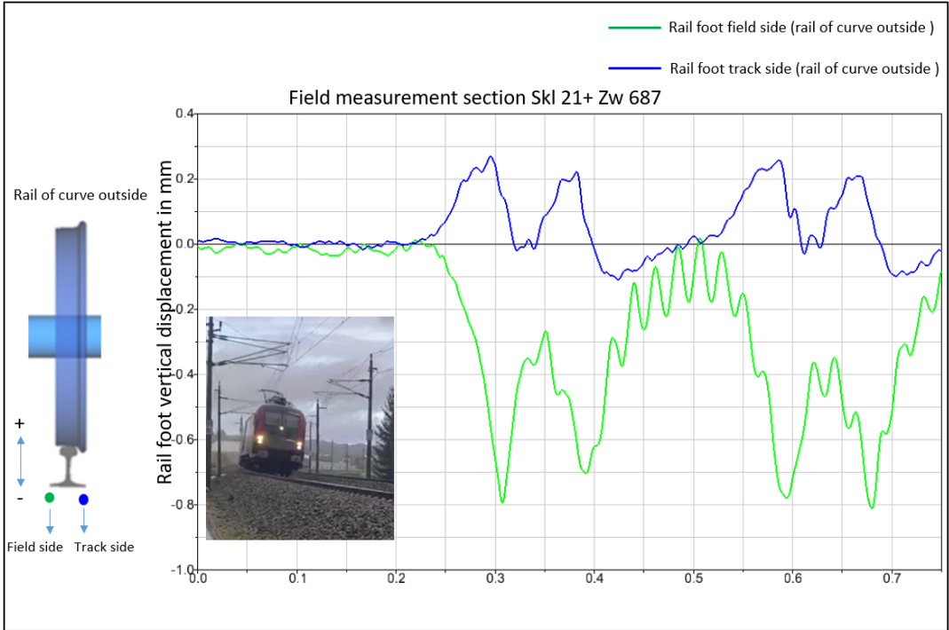
Figure: Rail foot vertical displacement measurement section SkI 21 + Zw 687
