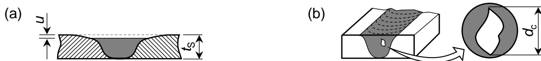
Figure 2.4: Schematic depiction of (a) a seam underfill and (b) a cavity (based on ISO 25239-5)
