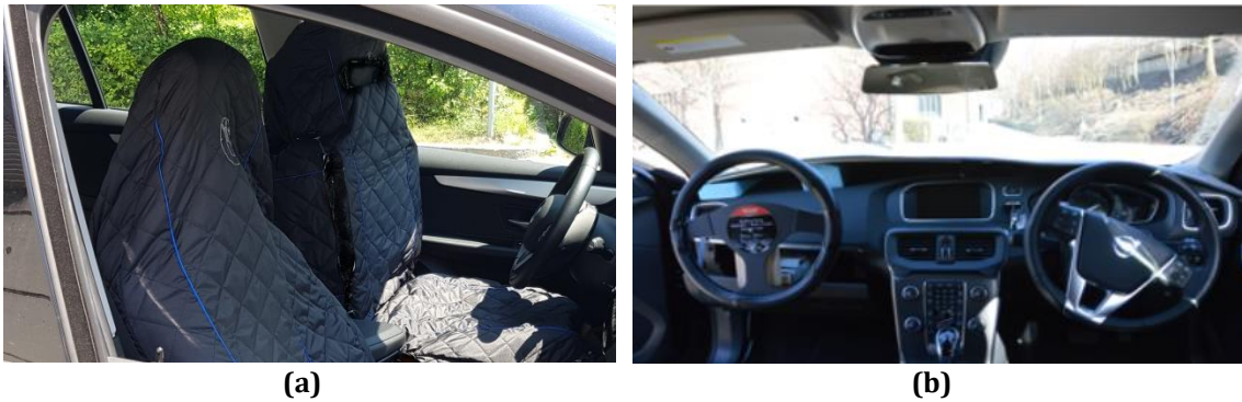
Figure 3.1 Wizard of Oz approaches: (a) seat cover (Fuest, Michalowski et al., 2019, p. 3955); (b) right-hand steered vehicle (Habibovic et al., 2016, p. 33).
