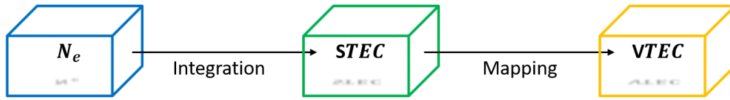
Figure 1.1: Relation between ionospheric key-quantities; the left part presents the integration of N_e along the ray path of a signal which leads to the STEC. The right part indicates a projection of the STEC into the vertical direction by means of a mapping function, leading to the VTEC.
