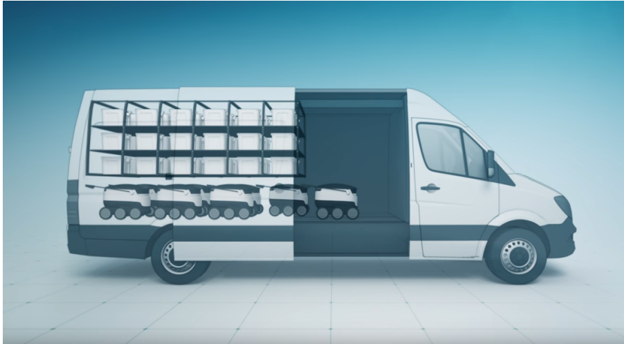
Figure 4.1: Specialized truck with freight containers and delivery robots (Mercedes-Benz Vans, 2016)
