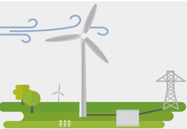
Fig. 3.2: Transformation of the wind flow into a renewable-energy form by converting the rotational motion of the turbine's blades into electricity using a generator Courtesy of NC Sustainable Energy association
