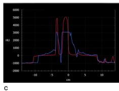
**Figure 4.** Differences in image quality for patients with metal implants using a kilovoltage CT (**a**) and the Radixact MVCT (**b**). Graphic (**c**) shows the Hounsfield unit (HU) comparison of image (**a**) in blue and image (**b**) in red. Obviously, densities with associated HUs above 3071 are not.
