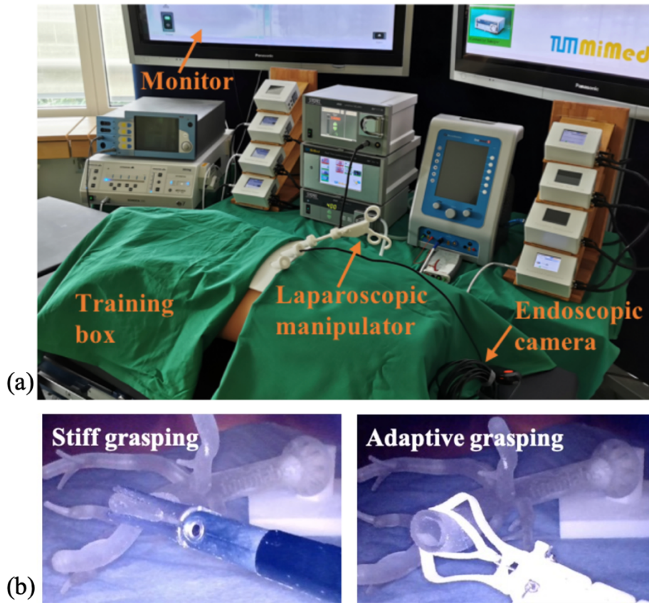
Figure 6-30: Endoscopic experiment in a training box: a) Setup of the test composed of a training box, an endoscopic camera, a laparoscopic manipulator and a monitor, b) Images taken by the endoscopic camera showing the grasping effect of the conventional and adaptive MIS forceps.
