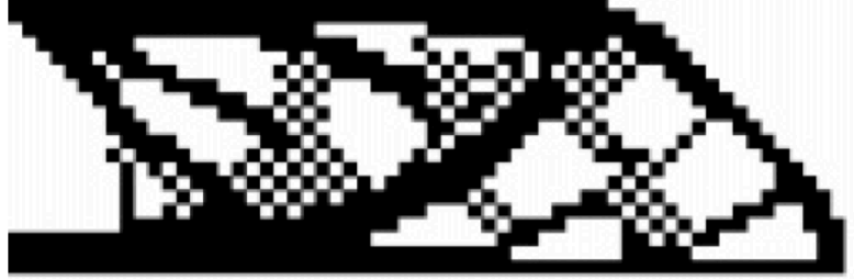
Figure 4-10: A topology optimized statically stable structure without filter (reproduced from Bourdin, 2001).
