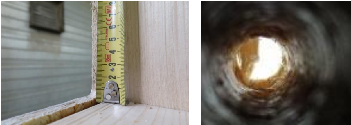
Figure 56: Left: Manual measurement of the module showing deviations between the frame and the board. Right: Deviation of the hole made on the board by the Weinmann and the hole made on the profile by the K2 Hunddegger.
