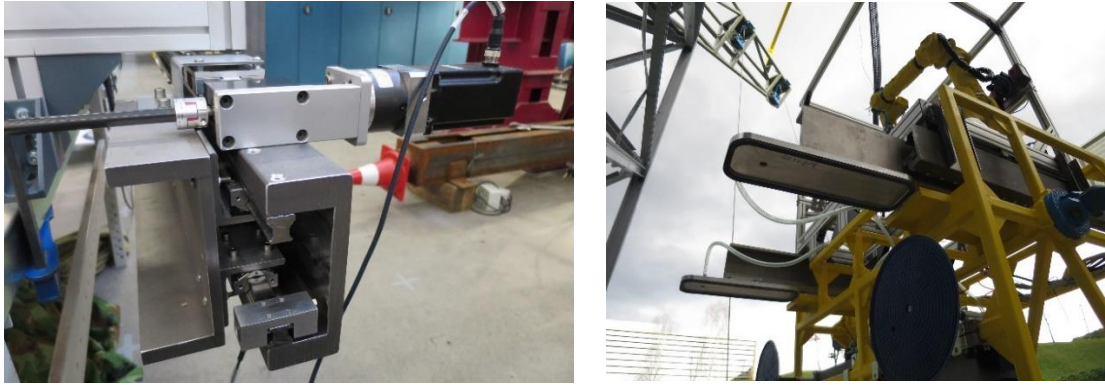
Figure 116: Left: the linear actuator solution in the lab. Right: the linear actuator performing on the prototype.
