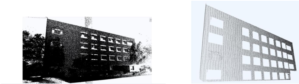
Figure 33: Left: merged Point Cloud of a building and surrounding area. Right: after processing.
