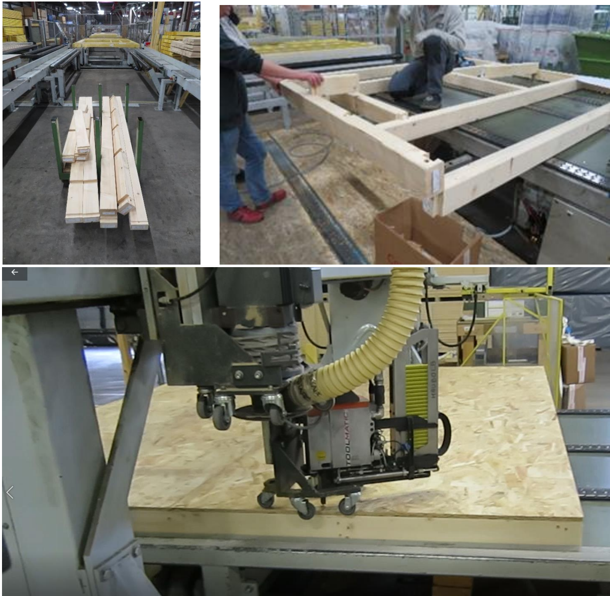
Figure 53: Top: handling the profiles to Workstation 2 and assembly of the profiles in Workstation 2. Below: nailing in Workstation 3.
