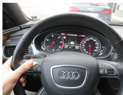
(b) Part II: Button at the steering wheel to start the lane change.
