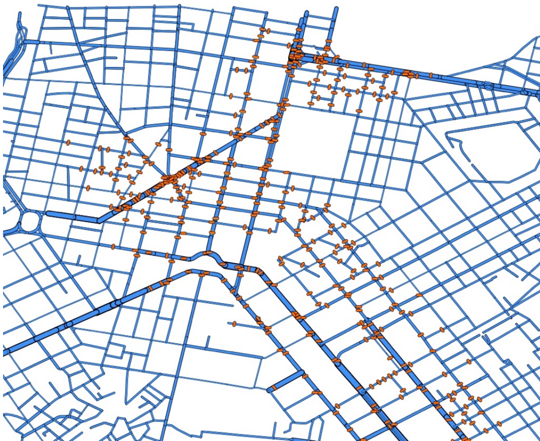
Figure 3.12 Result of virtual detector installation
