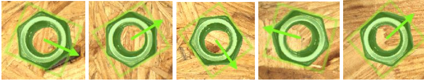
Figure 8.3: Example for classes without orientation. For a symmetric object like the shown nut, the correct orientation is ambiguous to annotate. Therefore, we assign it to be a class without orientation .
