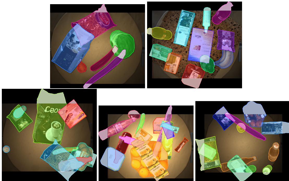
Figure 11.4: D2S amodal ground truth. Exemplary ground truth annotations for different splits of the D2S amodal dataset. Two images with different backgrounds from val (top), two generated images from augmented , and an image generated from modal annotations modal augmented (bottom, from left to right).
