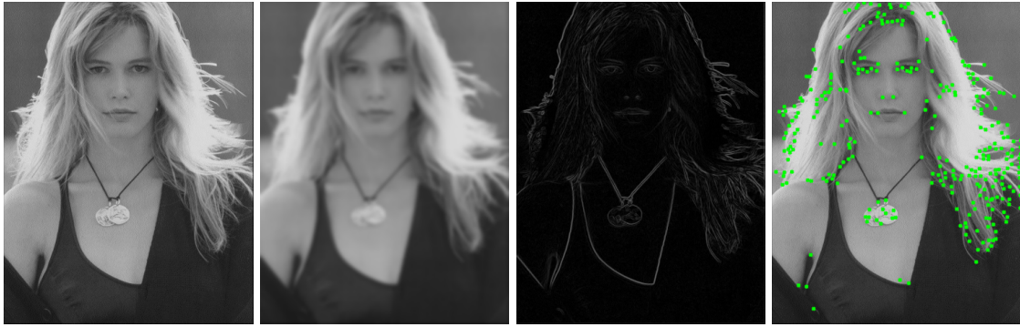
Figure 2.6: Filters and keypoints. (From left to right) The input image, and after a convolution with a Gaussian kernel of size 11 \times 11 . Edge amplitudes extracted with the Sobel operator. Keypoints obtained with the Harris corner detector.
