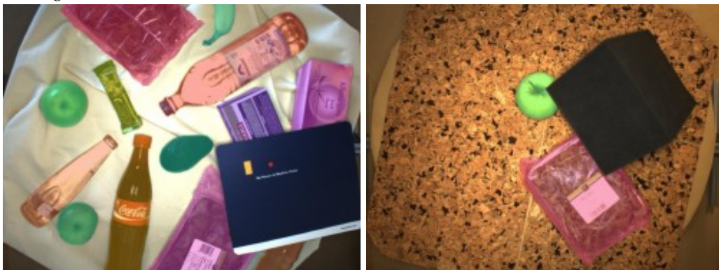
Figure 5.6: Clutter. To test the robustness of approaches to unseen clutter objects, objects not within the training set were added to the validation and test sets (e.g., a mouse pad and a black foam block).
