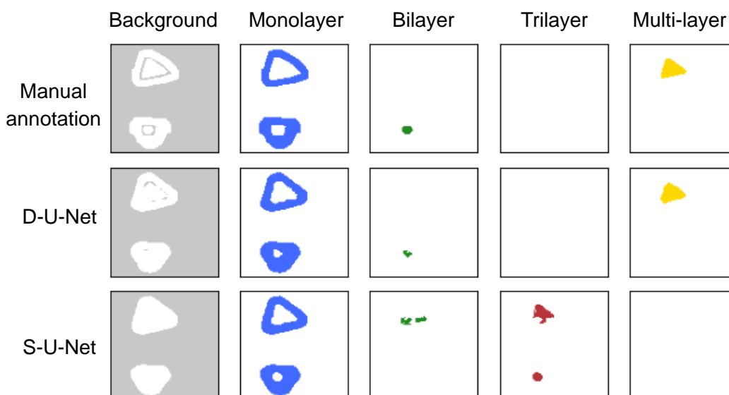
Figure 6.15: Prediction results of the distribution maps of substrate, monolayer, bilayer, trilayer, and multi-layer flakes by the deep fusion network and the single-stream U-Net (Figure 6.12 (c)).
