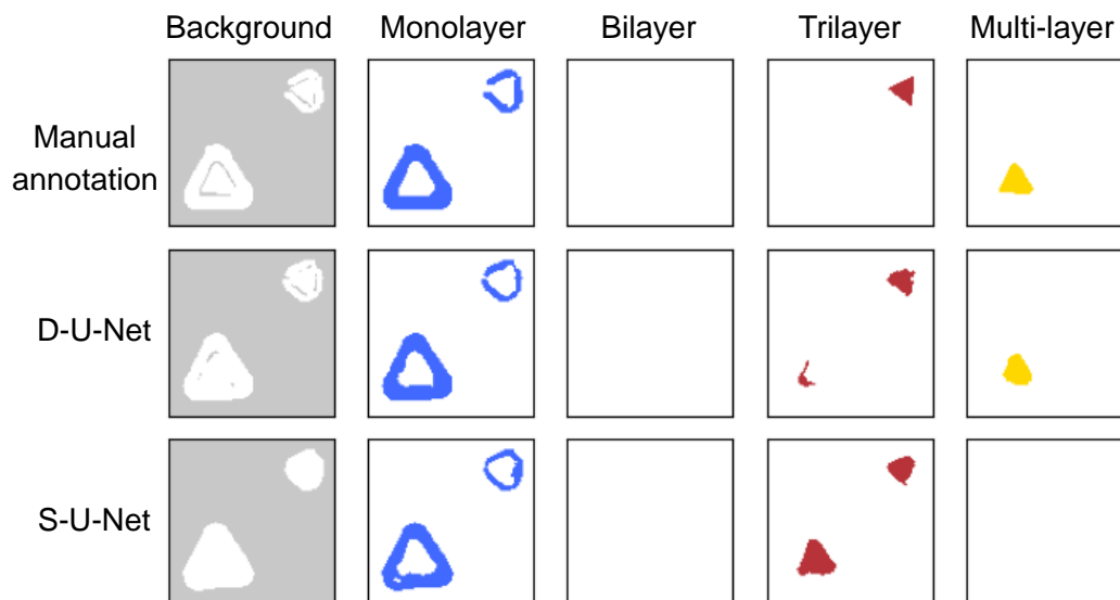
Figure 6.14: Prediction results of the distribution maps of substrate, monolayer, bilayer, trilayer, and multi-layer flakes by the deep fusion network and the single-stream U-Net (Figure 6.12 (b)).
