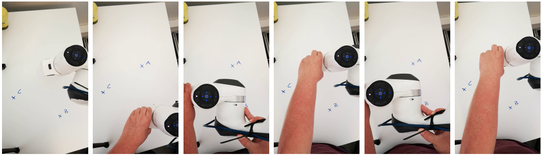
Figure 4.2: Illustration of the three point motion task execution. The robot is guided in two rounds over the three marked points (A, B, C). In the second round, point B is passed without stopping.
