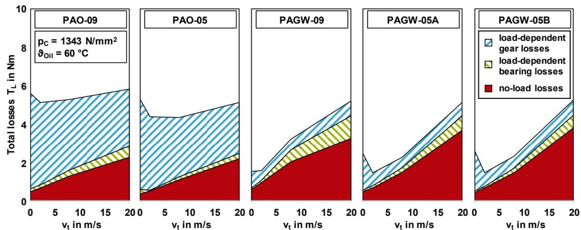
**Figure 3.** Total losses, no-load losses, load-dependent bearing losses, and load-dependent gear losses for  $p_c = 1343 \text{ N/mm}^2$  and  $\vartheta_{Oil} = 60 \text{ }^\circ\text{C}$  over the pitch line velocity  $v_t$  based on [16].
