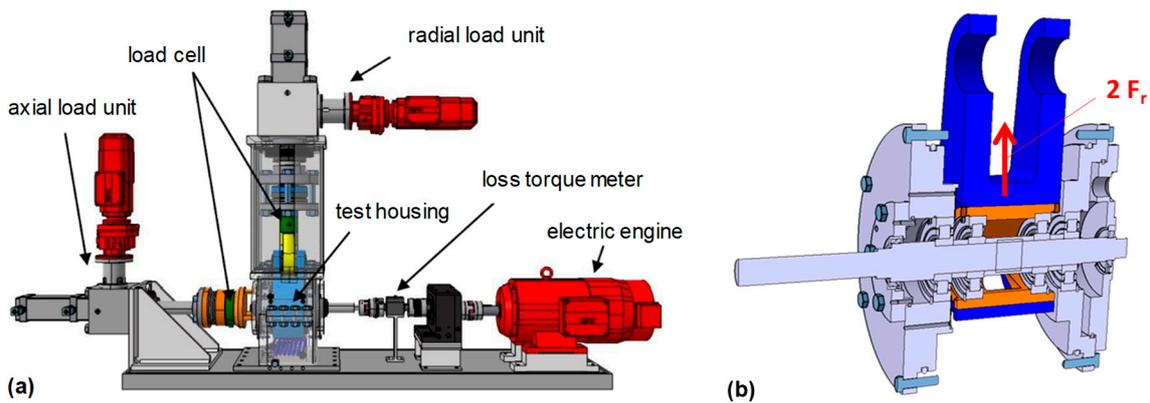
**Figure 1.** Mechanical layout of the FZG bearing power loss test rig (a) and assembly of the test bearings in the test housing (b) according to Jurkschat et al. [3,9].
