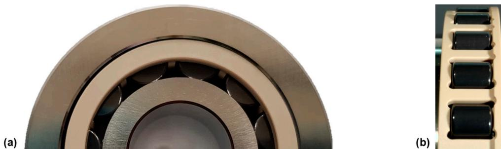
**Figure 2.** Type NU406 and NJ406 test bearings with common front view (a) and top view (b).
