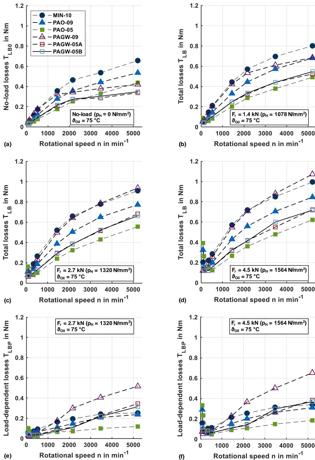
**Figure 4.** Measured no-load losses (a) and total losses for radial forces of  $F_r = \{1.4, 2.7, 4.5\}$  kN (b–d) as well as derived load-dependent losses for  $F_r = \{2.7, 4.5\}$  kN (e,f) over the rotational speed for all investigated lubricants ( $\vartheta_{oil} = 75\text{ }^{\circ}\text{C}$ ).
