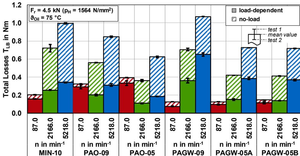
Figure 5. Influence of rotational speed  $n = \{87, 2166, 5218\} \text{ min}^{-1}$  on the measured no-load and derived load-dependent losses at  $F_r = 4.5 \text{ kN}$  and  $\vartheta_{Oil} = 75 \text{ }^\circ\text{C}$  for all investigated lubricants.
