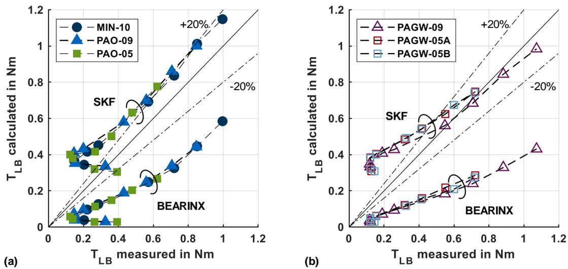
**Figure 7.** Comparison between calculated and measured total bearing losses  $T_{LB}$  at  $F_r = 4.5$  kN,  $\vartheta_{Oil} = 75$  °C and  $n = \{87, 131, 348, 522, 1444, 2166, 3479, 5218\}$  min<sup>-1</sup> for conventional gear oils (a) and water-containing gear fluids (b).
