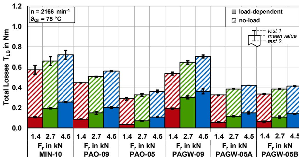
Figure 6. Influence of radial force  $F_r = \{1.4, 2.7, 4.5\} \text{ kN}$  on the measured no-load and derived load-dependent losses at  $n = 2166 \text{ min}^{-1}$  and  $\vartheta_{Oil} = 75 \text{ }^\circ\text{C}$  for all investigated lubricants.
