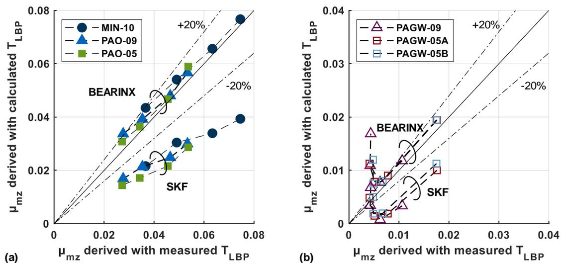
**Figure 8.** Comparison of derived mean gear coefficients  $\mu_{mz}$  with measured and calculated load-dependent bearing losses  $T_{LBP}$  at  $p_C = 1723$  N/mm<sup>2</sup>,  $\vartheta_{Oil} = 60$  °C and  $v_t = \{0.5, 2.0, 8.3, 20\}$  m/s for conventional gear oils (a) and water-containing gear fluids (b).
