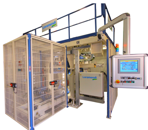
Figure 4.3: Loramendi core shooting machine SLC2-25L, which is utilised for the specimens of type IN-1 in this thesis.
