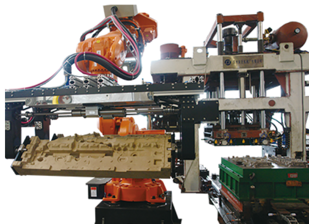
Figure 2.6: Core handling robot with specialised gripper (Muschna, 2020). In modern core production, cores often are handled with robots. Depending on the gripper and the geometry and the weight of the core, the stresses in the core are significant.
