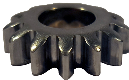
Figure 2.14: Fineblanked gear wheel with a distinct die roll.
