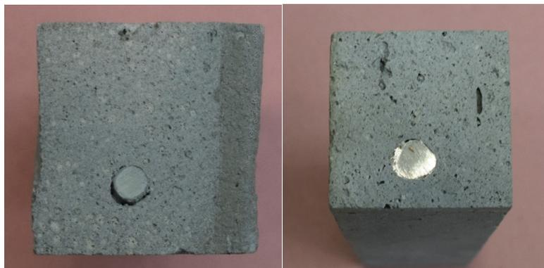
**Figure 16.** Bond between mortar and rebar: glass fiber (**left**), steel (**right**).
