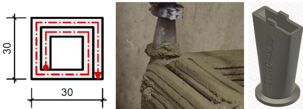
**Figure 2.** Sample geometriy (left), deposition of a layer on top of horizontal reinforcement (middle) and nozzle with tongue (right).
