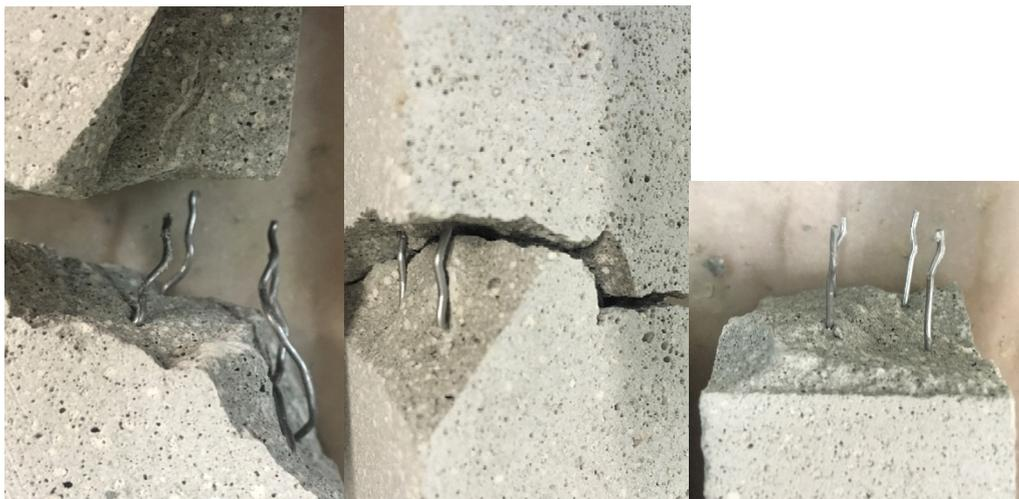
**Figure 18.** Fracture surface depending on the bond behavior.
