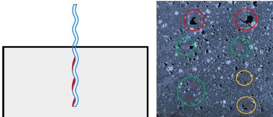
**Figure 17.** Schematic cavity formation around the vertically inserted fibers (left). Different quality of bond between fibers and mortar (right—red: bad, yellow: satisfactory, green: good bond behavior).
