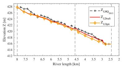
**Figure 14.** Longitudinal section of the maximum water surface levels: Observed in 2013 ( $Z_{f,HQ_{2013}}$ ), and simulated by the draft scenario ( $Z_{f,Draft}$ ) and the simulated optimised case ( $Z_{f,Opti}$ ).
