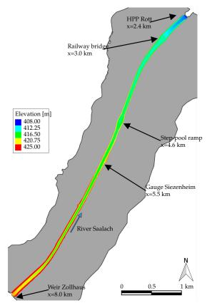
Figure 4. Extension of the original computational grid (grey) and the extracted main channel (colored).
