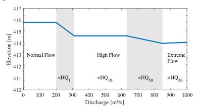
**Figure 3.** Stage-discharge-relation at the HPP Rott for the different operation modes and the transition zones.
