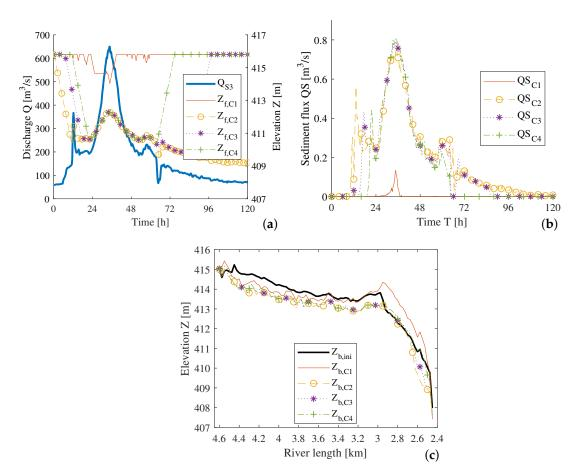
**Figure 10.** Extreme flood scenario: (**a**) boundary conditions for the extreme flood scenario and the four investigated regulation schemes; (**b**) simulated sediment flux at the outlet boundary for each case; and (**c**) longitudinal section of the mean riverbed in the reservoir for initial conditions (black) and the final situation for each case.
