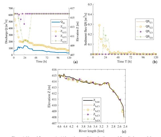
**Figure 8.** Normal flow scenario: (**a**) boundary conditions for the normal flow discharge and the water surface level of the four cases; (**b**) simulated sediment flux at the outlet boundary for each case; and (**c**) longitudinal section of the mean riverbed in the reservoir for initial conditions (black) and the final situation for each case.
