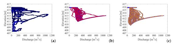
**Figure 12.** Stage-Discharge-relation for the three weir operating schemes: (**a**) observed; (**b**) draft; and (**c**) optimised.
