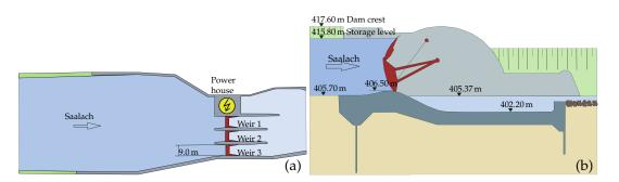
**Figure 2.** Simplified sketch of the HPP Rott: (**a**) top view, with the upstream reservoir, the weir with gates, and the orographically left located power house with the turbine intake; and (**b**) longitudinal section through one of the weirs.
