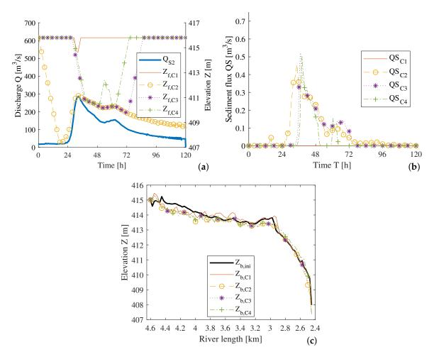
**Figure 9.** Medium flood scenario: (**a**) boundary conditions for the medium flood scenario and the four investigated regulation schemes; (**b**) simulated sediment flux at the outlet boundary for each case; and (**c**) longitudinal section of the mean riverbed in the reservoir for initial conditions (black) and the final situation for each case.
