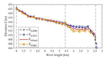
**Figure 13.** Longitudinal section of the riverbed levels: Observed in 2006 ( $Z_{b,2006}$ ) and 2013 ( $Z_{b,2013}$ ), as well as the result of the draft scenario ( $Z_{b,Draft}$ ) and the simulated optimised case ( $Z_{b,Opti}$ ).
