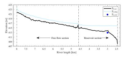
**Figure 5.** Longitudinal section of the initial bathymetry of the Saalach River, representing the maximum acceptable riverbed in the reservoir  $Z_{b,ini}$  (**black**), the water surface level  $Z_{f,MQ}$  (**light blue**) during normal mean discharge conditions, and the top edge of the ground sill  $Z_{b,GS}$  at x = 3.0 km.
