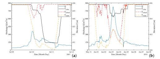
**Figure 11.** Hydrograph and corresponding water surface levels for sediment-flushing for the observed (black), the draft (red) and the optimised (orange) scheme for two time periods: (a) July 2007; and (b) June 2010.
