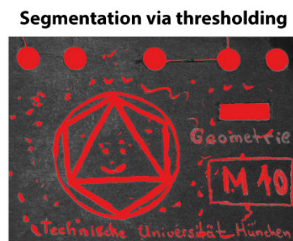
Fig. 3.11. Segmentation clutter. The task is to mask the discs in the upper part of the image. The proposed segmentation pipeline alone is incapable of removing the clutter in the background and thus the mask shown in red contains more pixels.
