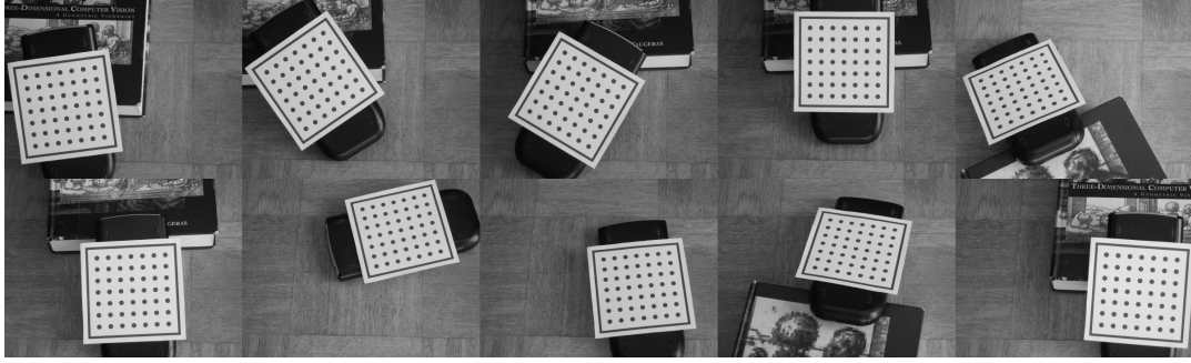
Fig. 4.11. Multi-image calibration. Each acquisition gives a set of 49 co-planar points together with 6 extrinsic parameters. Multiple images increases the amount of data points for our optimization problem. The intrinsic parameters remains the same while the extrinsic values vary between different acquisitions.
