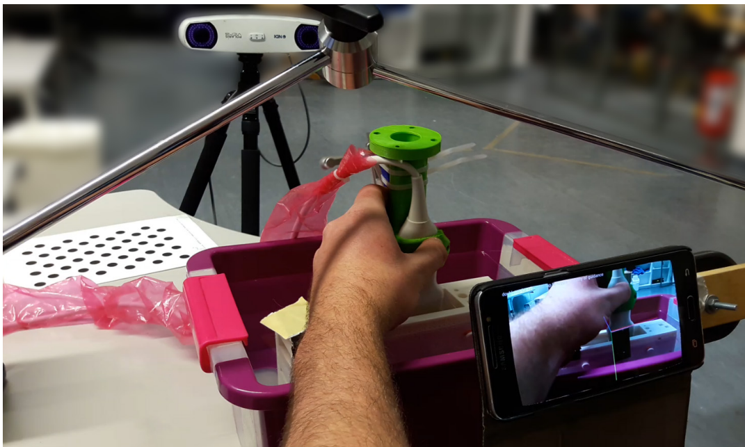
Fig. 7.6. Mobile augmented reality. An optical stereo tracking system (top, white) tracks both the rigid body marker attached to the green mount of an ultrasound transducer (centre) and a spherical marker frame on a wooden bar (right) where a mobile phone is fixed. All sensors are co-calibrated such that the live ultrasound video can be sent wireless to the mobile phone together with the correct pose such that it can be rendered at the current position on top of the RGB video stream of the mobile camera. A 3D coordinate frame additionally visualizes the live ultrasound coordinates.
