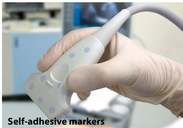
Fig. 7.5. Tracking marker comparison. A rigid body marker with four exchangeable spheres is shown on top left. Despite their size, these are usually attached to medical instruments (top right). Self-adhesive markers (bottom) with 5 mm diameter allow for intuitive use of the medical instrument while generating a multi-redundant cue for an optical tracking algorithm.
