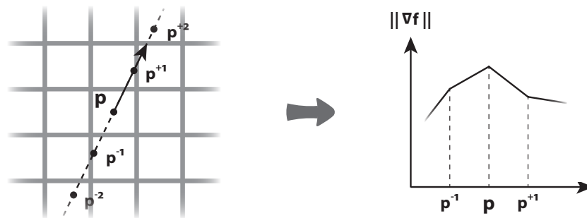
Fig. 3.26. Edge detection with interpolation along gradient direction. On the left, the gradient \nabla f(p) at p (visualized with an arrow) is used to calculate the direction which is illustrated as a dashed black line. Samples along the line are taken at discrete steps forwards (+) and backwards (-). The right graphic illustrates the interpolated gradient magnitude for some example locations.
