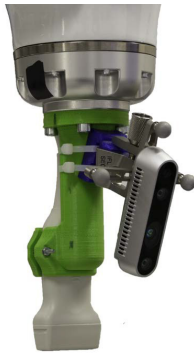
Fig. 7.34. Dynamic OTS prototype evolution. The first dynamic OTS systems (top left) are a direct integration of the marker-based outside-in concept with a significantly smaller size such that they can be mounted on a robotic arm. A second iteration (top right) leaves out the ring LED lights to enable a passive stereo system with similar geometry. In order to miniaturize and enable mobile hand-held applications for inside-out usage, an RGBD sensor is used (bottom). A boxed version based on an intel RealSense D435 camera with the dimension of 90 mm x 25 mm x 25 mm is used with a flexible mount (bottom left). It is further miniaturized with a board-level version of the intel RealSense D430 (bottom right).
