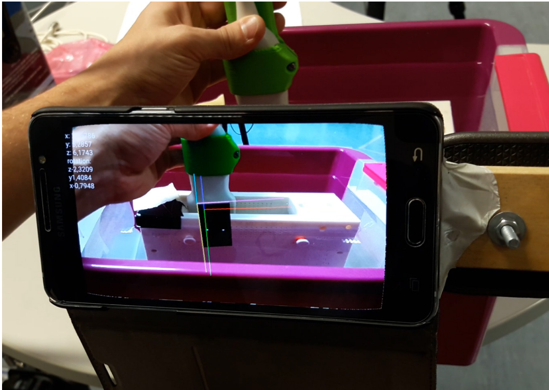
Fig. 10.7. Experimental setup for wire phantom alignment. The mobile phone is fixed in front of the phantom while the user is asked to align the ultrasound image with a plane given by two wires inside the water bath. The numerical values (top left of the screen) show the deviation from a target helper pose which is augmented here (red-green-blue) in comparison with the current pose (magenta-yellow-cyan). The current ultrasound image is overlaid as anatomical guidance.
