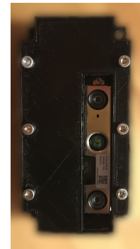
Fig. 7.34. Dynamic OTS prototype evolution. The first dynamic OTS systems (top left) are a direct integration of the marker-based outside-in concept with a significantly smaller size such that they can be mounted on a robotic arm. A second iteration (top right) leaves out the ring LED lights to enable a passive stereo system with similar geometry. In order to miniaturize and enable mobile hand-held applications for inside-out usage, an RGBD sensor is used (bottom). A boxed version based on an intel RealSense D435 camera with the dimension of 90 mm x 25 mm x 25 mm is used with a flexible mount (bottom left). It is further miniaturized with a board-level version of the intel RealSense D430 (bottom right).
