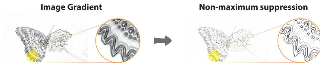
Fig. 3.28. Image gradient before and after non-maximum suppression. The left image depicts the image gradient and a magnification. Note the spurious points. After edge thinning with non-maximum suppression, the contours are more clearly defined as shown on the right.
