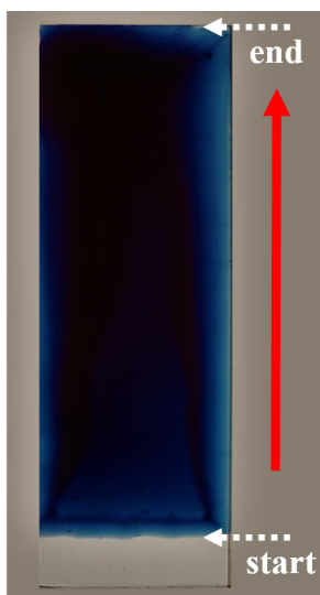
Figure 4.3: Photograph of a slot-die coated active layer based on PBDB-T-SF:IT-4F printed out of CB on a glass substrate (7.5 cm × 2.5 cm). The start and end position are labeled with white arrows. The printing direction is indicated by a red arrow. Reproduced and adapted with permission from ACS publishing [243].
