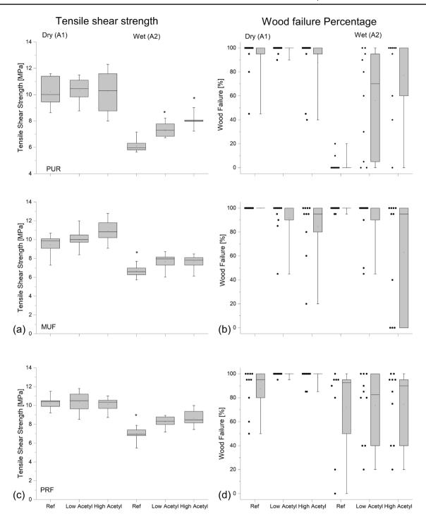
**Fig. 4** Comparison of the effects of the level of acetylation on tensile shear strength  $(\mathbf{a}, \mathbf{c}, \mathbf{e})$  and wood failure percentage  $(\mathbf{b}, \mathbf{d}, \mathbf{f})$  of rubberwood bonded with PUR  $(\mathbf{a}, \mathbf{b})$ , MUF  $(\mathbf{c}, \mathbf{d})$ , and PRF  $(\mathbf{e}, \mathbf{f})$  during test in dry (A1) and wet (A2) conditions. For wood failure  $(\mathbf{b}, \mathbf{d}, \mathbf{f})$
