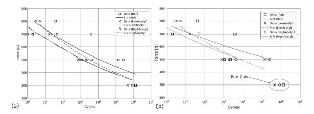
**Fig. 5** Simplified S–N curves for Ref, LowAcetylated and HighAcetylated samples bonded with PRF. These S–N curves are obtained according to a power model (P<sub>max</sub>=bN<sup>a</sup>), with **a** run-out samples being considered as fractured samples and included in the regression
