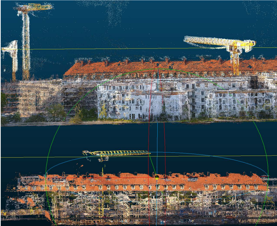
Figure 4.6: Point-clouds from automatic reconstruction (up) and DSP version (down) locate different and have different directions in one coordinate system.
