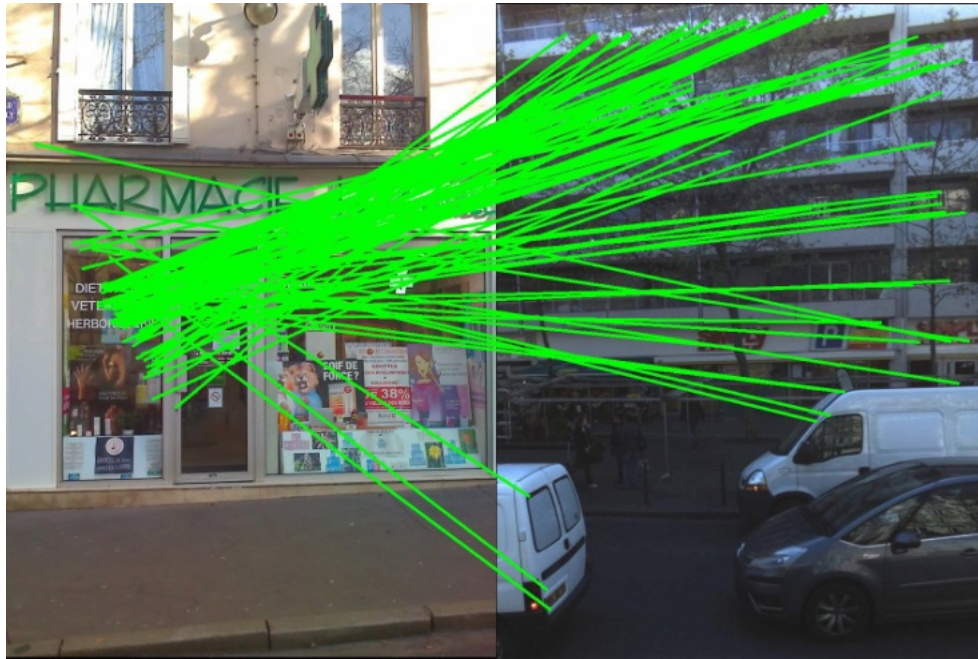
Figure 2.11: Non-discriminating features like from tree branches disturb the matching.
