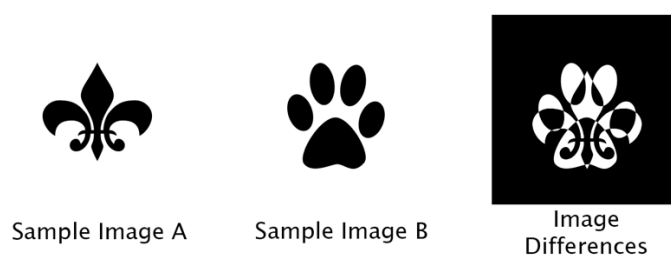
Figure 2.3: An intuitive illustration for image subtraction. Black for same pixels and white for difference.
