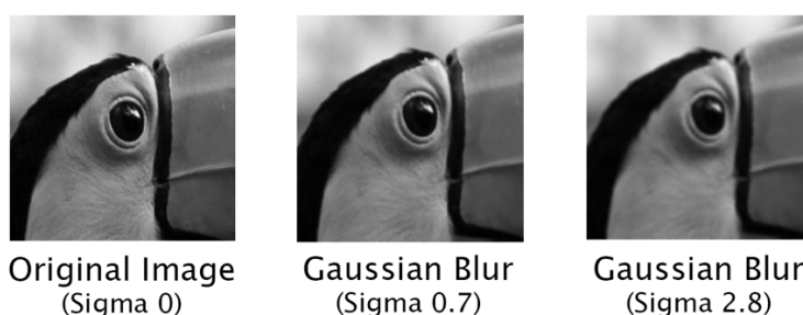
Figure 2.1: A set of images blurred with a Gaussian Blur at different sigma. [10]
