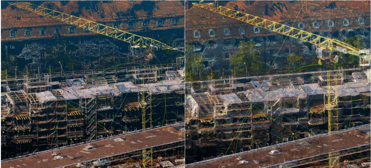
Figure 4.13: Point-clouds with window radius of 2 (left) and 14 (right).
