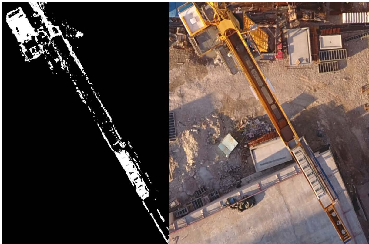
Figure 5.1: Bad reconstruction in the shadows (geometric depth-map).
