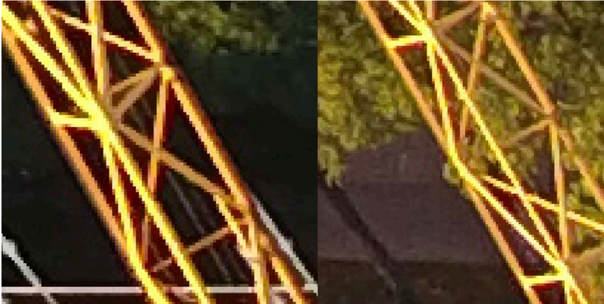
Figure 5.3: Visible purple fringes on the edge of the crane elements.
