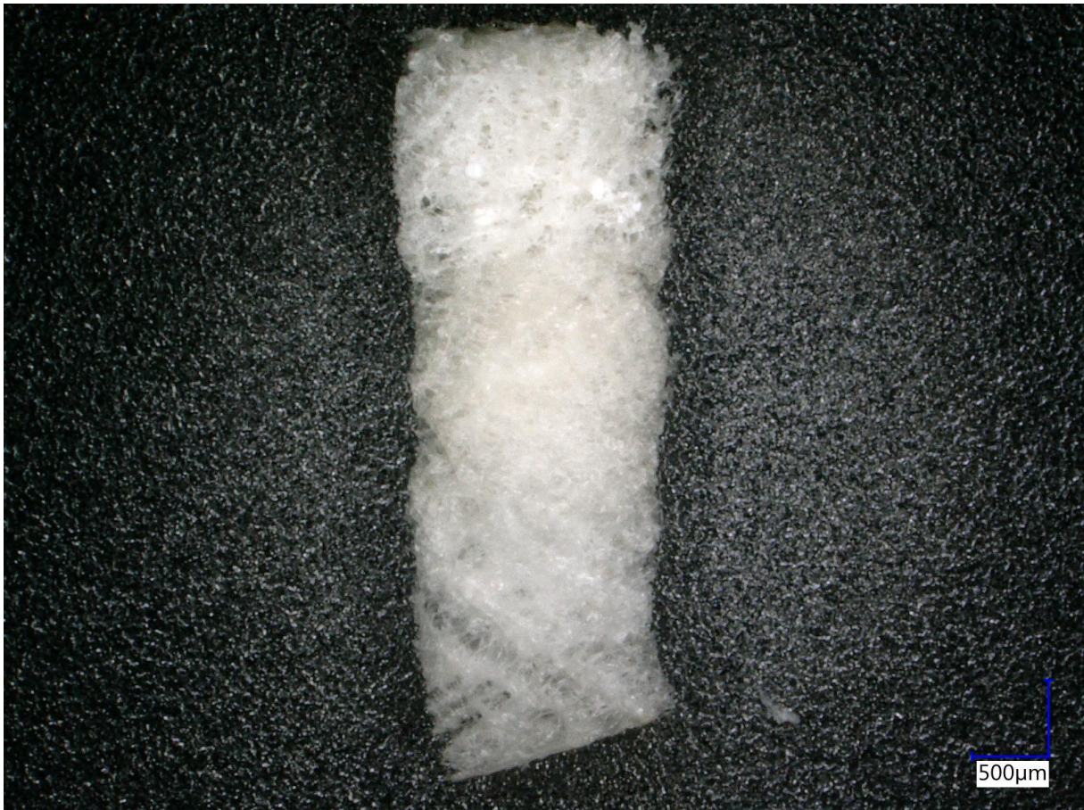
Figure 2: Digital microscope picture with full depth of field of 3-layered scaffold
