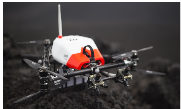
FIGURE 1 In-house built hexacopter autonomous robot design for extraterrestrial application on Mt. Etna. Its size and weight is 68 \times 68 \times 30 cm and 2.65 kg, including battery, respectively [Color figure can be viewed at wileyonlinelibrary.com ]
