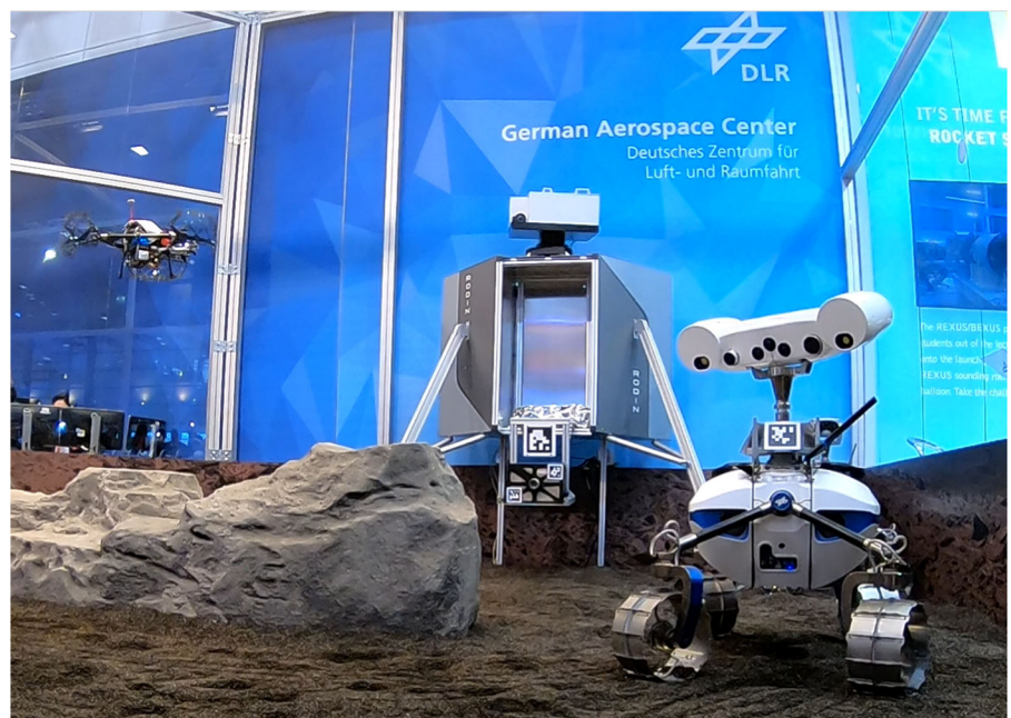
FIGURE 25 ARDEA and LRU perform an exploration mission at the IAC 2018. One laser terminal is mounted on the top of the lander mock-up in the back [Color figure can be viewed at wileyonlinelibrary.com ]
