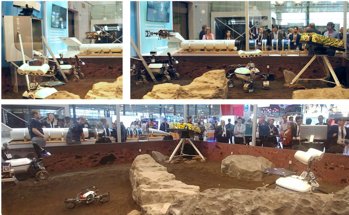
FIGURE 26 Impressions of our cooperative multirobot mapping demonstration at the IAC 2018 with a heterogeneous team of rover and hexacopter: ARDEA observing LRU from its first waypoint after takeoff from the rover’s transport platform (top left), ARDEA on its return flight while LRU is navigating to the location explored by ARDEA. One laser terminal is visible on the right side (top right), and ARDEA landed next to its start position while LRU reached its target destination (bottom) [Color figure can be viewed at wileyonlinelibrary.com ]
